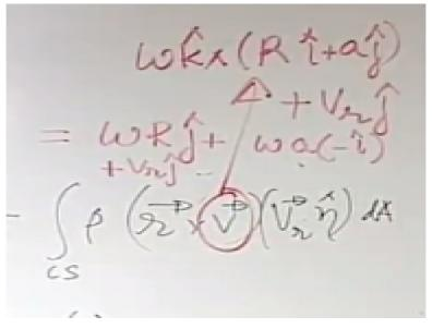
So, that is omega r square K then, so you write this as omega r square then in place of dV, A dr this thing K, right then plus, again you assume uniform velocity distribution, so when you write the next term, then what should you substitute for this V? This one; yes, remember this V has to be inertial reference frame V, so what is that? So, omega K cross with capital ri + aj + Vrj, right, so what will be that? Omega rj + omega a - i + Vrj.
