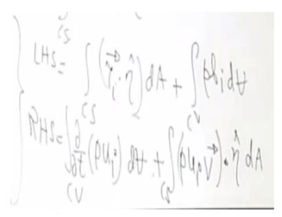
So, this of rho ui, this V is replaced by its component along i and then the remaining integral of rho, this V is replaced by ui, okay, the next steps are quite simple, the next steps are converting the area integrals into the volume integral, so that we may convert all the area integrals into the corresponding volume integrals.
