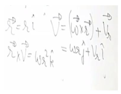
This is velocity of the solid plus velocity of the fluid relative to the solid, so what is the velocity of the solid at the coincident point at a radial location r, it is omega cross r, so this is the velocity of the solid plus the velocity of the fluid or V relative or Vr, so this is omega rj+Vri, right. So, we substitute that but before substituting maybe it is useful to find out how it is r cross V.
