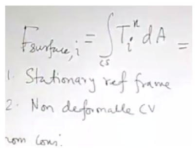
So, you should make the all the terms compatible for use of the divergence theorem, all the area integral terms at least. So, when you are trying to represent the surface force, what is the surface force, F surface is? F surface i, so let us just write the i component, x component, so when we call the components will not put a vector sign because the components are just the scalar components.
