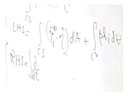
If you integrate it over the control volume, it will give the total body force along i, okay, so we have been successful in writing the left hand side in a certain way for force components along i, so the left hand side will become integral of over the control surface tau i dot with eta dA + control volume rho Vi dV, what about the right hand side? We will take the time derivative term inside the integral because of non-deformable control volume.
