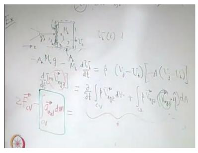
Let us say that there is a block, which is moving on a surface or which may move on a surface from a nozzle a water jet comes strikes this one and gets deflected in the two sides
