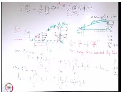
Fluid is coming from height stream with a uniform velocity say u infinity. This fluid is falling on the plate and because of its viscous interactions the effects of viscosity within the fluid. The first thing is the plate tries to slow down the fluid which is in contact with that and that effect is propagated to the outer fluid through the viscosity of the fluid. There is a thin layer close to the wall where this effect of the plate is felt and the velocity gradient is created.
