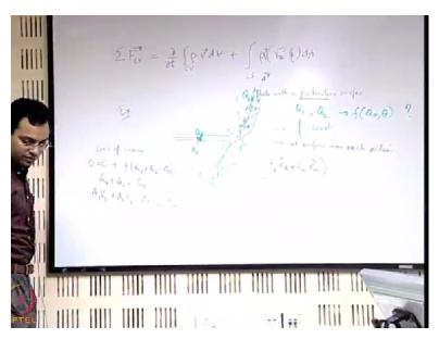
Which comes out of a tube or may be a small pipe and say there is a plate which is frictionless and oriented inclined to the jet this is a plate with the frictionless surface. So, what happens to the water? The water extreme stream lines come like that and water leaves across the ends of the plate this way. We have to find out if the volume flow rate here is Q0 and here the volume flow rate is Q1 and if the volume flow rate Q2.
