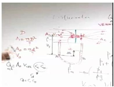
So we can say that the final expression is you have Q= A0 \*Vc theoretical both of which you have determined A0 you know area of the orifice. You know the Vc theoretical from this simple analysis multiplied by CC \* Cv. And this we call as Cd here coefficient of discharge. So this is the sort of ideal flow rate, but the thing is this be different from the previous case because in this case the areas and velocities are referred to 2 different sections.
