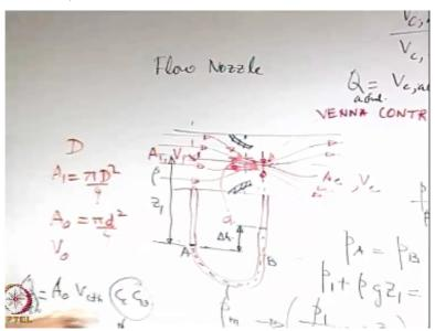
So what is a flow nozzle. We will not go into the detail construction of a flow nozzle. We will just try to go through the philosophy because it is something in between the venturimeter and orifice meter. It is the cost is in between the accuracy is also in between. So what it does is instead of putting a sharp orifice with an abrupt change puts a kind of nozzle at the wall. To have a more gradual change of the cross section of the area.
