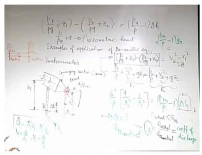
So if you recall what was the purpose of the venturimeter. The purpose was to measure the volume flow rate through a pipe. Now for that we utilize this type of an arrangement where you have a converging section which is sometimes also called as a converging cone. Then you have a throat where the area of cross section of the entire arrangement is a minimum and then a diverging section and the purpose is obvious that this part has to fit with the pipe.
