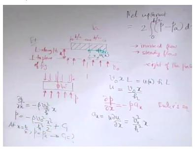
We refer to this example as such to work out a problem in the context of fluid kinematics. There is something like plate a rectangular plate and there is a bottom plate there are holes in the bottom plate through which fluid air is blown like this. If you recall, you walked out such a problem. And the velocity-- we will continue with that problem and try to work out a different problem on this.
