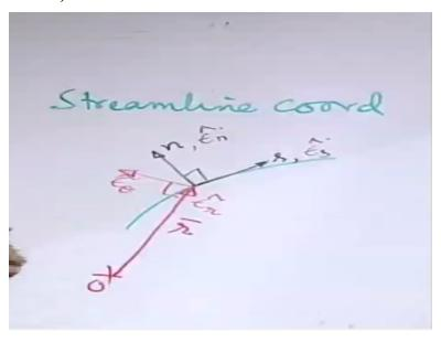
So if you have a streamline we consider tangential to the streamline as s and normal to the streamline as n. Okay. Many times there is confusion between these coordinate systems and the coordinate system that is used in a cylindrical polar coordinate system. So we will try to avoid that confusion from the very beginning. Say, if you are using a polar coordinate system. So if you have this as the origin of the pole then what how the coordinate is represented?
