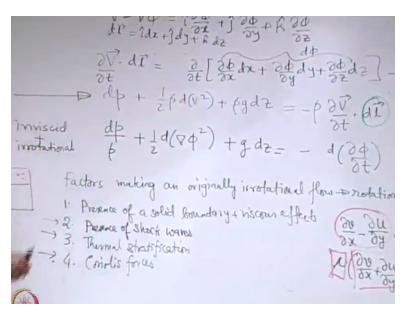
Example 3, Irrotational flow. So when you take the example of irrotational flow let us see that what happens to the equation. So when you have the irrotational flow the thing is that dl we are not writing as ds because when we are writing irrotational flow we are keeping in mind that it points 1 and 2 are taken such that they need not be along the same streamline. So if they need not be along the same streamline what is the consequence?
