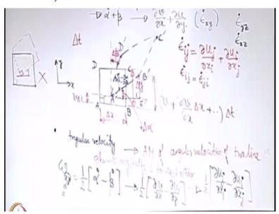
Why it is not so straightforward let us try to see, angular velocity. See whenever you were thinking of angular velocity, we were discussing about the rigid body motion but that is the special case. Usually, fluid is not under a rigid body motion just like this case. So when it is not in a rigid body motion you cannot really have a unique angular velocity of all the line elements in the flow.
