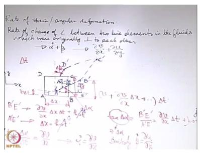
So to have a more formal definition we may say that we are defining the rate of strain or the rate of deformation in the following way. Rate of strain or angular deformation in what way? See there is a very important quantification of the distortion in the angle. What is that? If you consider 2 line elements AB and AD, they were originally at an angle 90 degree with each other.
