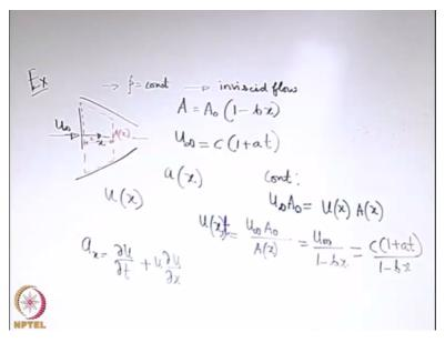
So we have a nozzle like this and it is carrying a fluid with density=constant and some other input data are given for the problem. The area of the cross section of the nozzle, it varies with area of the cross section of the inlet in the following manner where x is the coordinate measured from the entrance and other information that is given that the velocity at which the fluid enters the nozzle let us say that is u infinity that varies with time.
