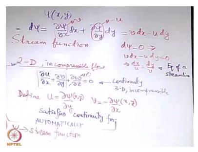
So stream function is defined as follows. To look into the definition let us first figure out that what is the motivation behind defining such a function. Let us take an example of 2-dimensional incompressible flow and write the form of the continuity equation for that. What is the form of the continuity equation for 2-dimensional incompressible flow?
