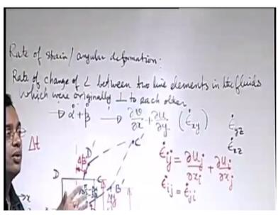
So this we may call as say epsilon dot xy as a symbol, epsilon for strain, epsilon dot for rate of strain, xy to indicate that it is actually an angular strain in the xy plane that is just a nomenclature. One may use of course different nomenclatures but I mean these also works. In this way, it is possible to write epsilon dot yz and epsilon dot xz. You see that specification of this epsilon dot requires 2 indices.
