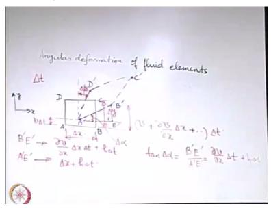
For the angular deformation, we will try to first sketch that how a fluid element when deformed angularly will look and then try to quantify it in terms of the velocity components, so angular deformation of fluid elements. Let us say that we start with rectangular fluid element like this. When we are thinking about angular deformation, the deformation is in terms of change of an angle and that angle change may take place in a plane.
