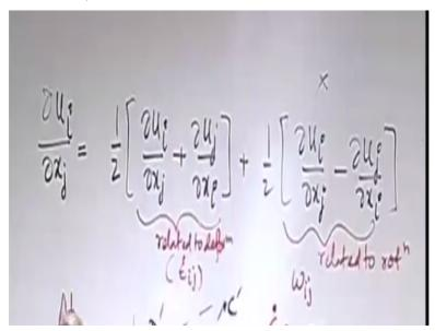
That is if you write the partial derivative of ui with respect to say xj, you can write it as this one plus of. Why it is important because this is a general velocity gradient and a general velocity gradient is what is related to what is expected to be related to deformation. Now you see that when you have a general velocity gradient out of that only one part is related to deformation and another part is not related to deformation.
