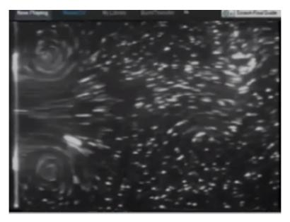
When you have these particles put in the flow and those particles are in forms of beads, so you can see that nice rotating structures or vortices can be observed with these particles, so these are called as streaks and we will see that why these are called as streaks.
