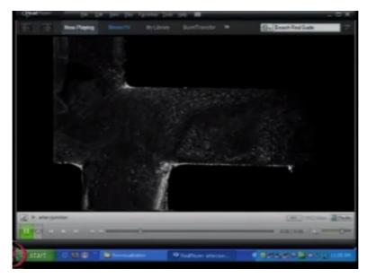
See this first example, so in this example, it is like flow in an artery junction, so there are certain tracer particles, so how this flow is visualized? You have tracer particles, so these particles may be very small beads of maybe nano meter size or few micron size and these beads are put in the flow and the flow is illuminated by say a laser source, so in that illuminated condition when the particles are moving, it is possible to not track individual particles all particles as such.
