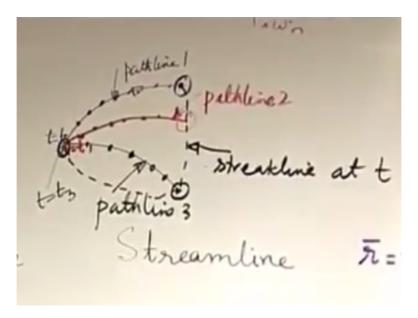
So, when we want to draw different path lines see at say time t = t0, you have one fluid particle which pass through this point of dye injection that fluid particle at subsequent instants of time, it is passing through different points, so this is the path line 1 say, what is that path line 1? Path line 1 is the path line of a fluid particle, which pass through the point of dye injection at time = t0.
