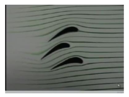
Let us look into a stream line example, so these are 3 cylinders in a steady flow and you can see that this green colour dye is giving an appearance of a stream line. Fundamentally, this is actually a streak line but because it is a steady flow, stream line, streak line, path line these are all identical, so these represent different streak lines or different stream lines or different path lines whatever you say, if it is a steady flow.
