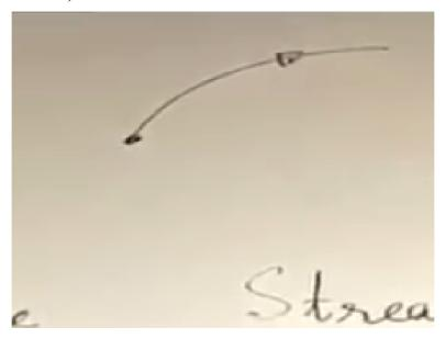
Let us try to conceptually draw a streak line, let us say that this is a point at which dye is injected, so when a fluid particle passes through these points say, at time = t0, so when at time = t0, the fluid particle passes through this point, the fluid particle then undergoes a locus. So, what is this locus?
