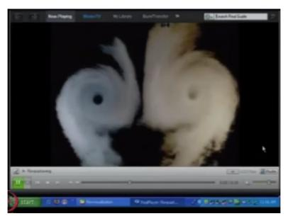
Now, we will not go into such analysis for this elementary course but if you just try to look into some other examples, this is particle visualization, this is also particle based visualization but visualization through smoke emission, so you can clearly see basically a wing of aircraft has passed and when it has passed, it has created a vortex, see the rotations and by the smoke emission that is being visualized.
