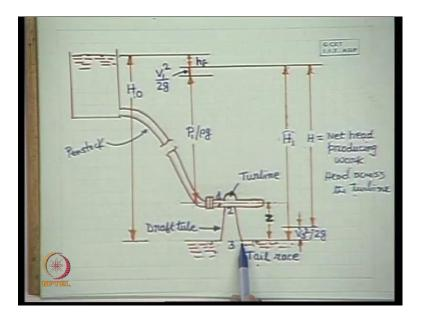
And a this is, because when the flow changes from section to section the flow velocity along with that the velocity of providing a draft tube a clear idea of the working principle of the draft tube. Now let us consider a very simplified diagram which will give you a clear concept of the change of head across the turbine.
