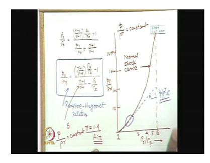
So, it is simply algebraic manipulation by which we get the density ratios after, and before shock in terms of pressure ratios or equating the pressure ratio finally, we can tell the pressure ratio in terms of the density ratio; that means, this is simply the manipulations of these equations; that means, here using the equation of state earlier we derived row y by row x as a function of mach number before the shock m a x.
