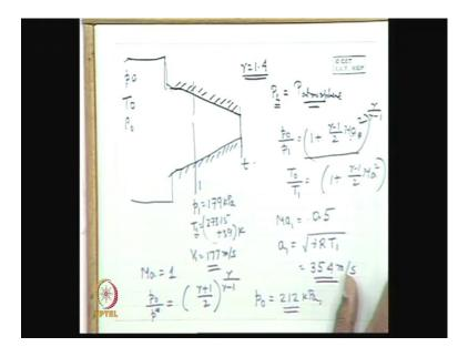
Let us find out that this is a problem converging nozzle is there. So, this is the discharge plane 1 thing is that it is discharging into atmosphere; that means, p b is p atmosphere now we do not have to be bias either way.
