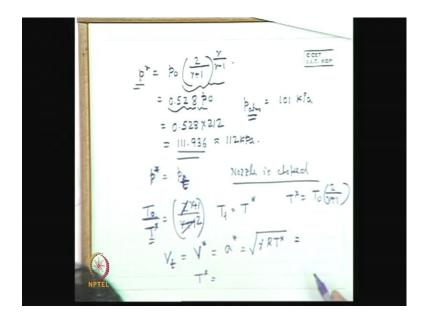
Which means that we can write this thing p star is equal to p 0 2 by gamma plus 1 by gamma by gamma minus 1, and this quantity with k gamma is equal to 1 point four is point five 2 eight this quantity is point five 2 eight of p 0 with gamma is 1 point four.
