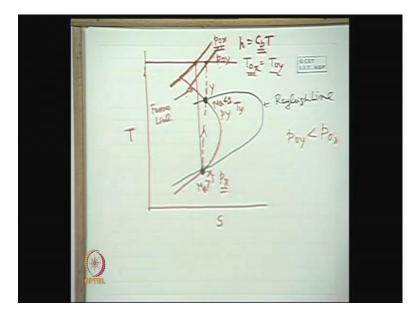
So, this is the change in entropy, now we just show at the end the come to this to have an idea o stagnation pressure temperature let us draw the fance line in t s diagram we know that we drew fance line earlier in h s diagram in a perfect gas h is equal to c p t for a calorically perfect gas c p is constant. So, h, and t are same; that means, they are just changed with a scale factor. So, the same graph we can draw in t s diagram with the
