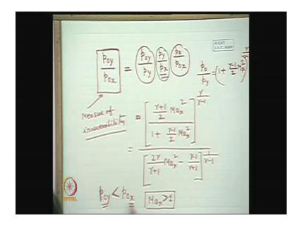
Now, 1 important thing is the stagnation pressure p o y, and p o x now see in a shock p o y, and p o x are not maintained same this is, because shock is an irreversible process friction is there. So, stagnation pressures are not same later.
