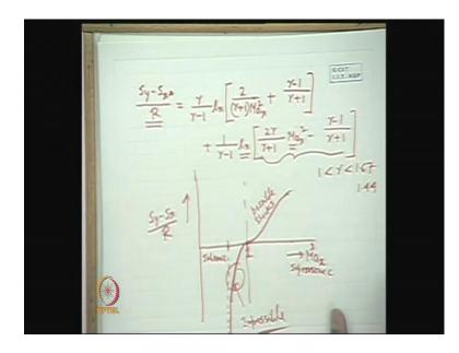
But if we want to express in terms of mach number at the upstream section m a, then we have to substitute this ratio as a function of m a which we have deduced earlier, and final result is that s y minus s x by r is equal to is a very big 1 gamma by gamma minus 1 there is no reason to remember it, but you must know this gamma plus 1 m a x square plus gamma minus 1 by gamma plus one.
