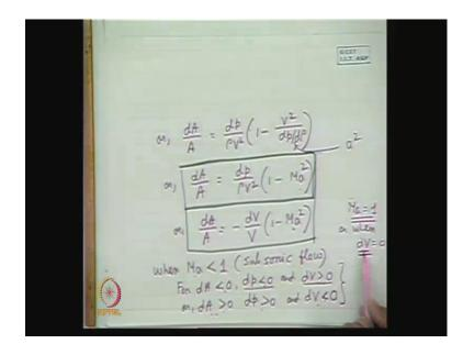
And next we can wire this d p by rho this we can write d p, if I take this d rho by rho d a by a d a by a in one side we can write d p by rho v square minus d rho by rho or we can write d a by a or or we can write is equal to d p by rho v square we take as common d p by rho v square into one minus v square divided by d p by d rho. So, again we can write d a by a or is equal to d p by rho v square, now what is this value d p by d rho in an isentropic flow.
