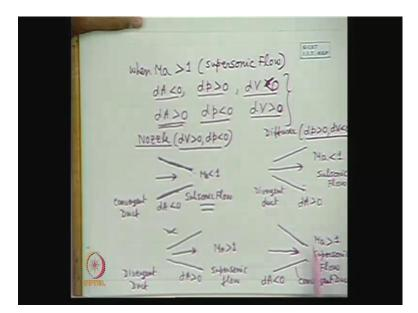
When just the reverse you see when mach number is greater than one that is supersonic flow supersonic flow you just see from the equation, when mach number is greater than one we see that when d a is less than zero d p is, because this is negative mach number greater than one.
