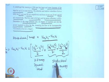
Now, with this I will go on solving a problem. Let us see this problem, a centrifugal fan ok a centrifugal fan running at 1500, that is fifteen hundred r p m, as inner and outer diameter of the impeller as 0.2 meter and 0.24 meter that is the inner diameter of the impeller, outer diameter of the impeller.
