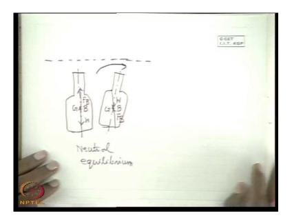
Now, the last possibility is the possibility, that G and B coincides, that means, this is the case when the weight, sorry, mass of the liquid is distributed, this is G, uniformly over the entire volume. That means, the weight acts to the center of gravity and the same point is the center of buoyancy, that is, F B. That means, the mass is uniformly distributed over the entire body. In this case, it is just like neutral equilibrium, as I have told earlier.
