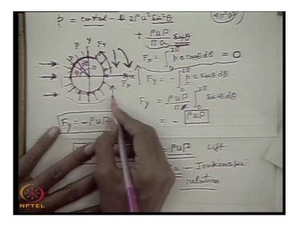
And this force is known as lift force, if it is in the upward direction. So therefore, you see that depending upon the direction of the vortex motion there is a direction of the transverse motion is created depends. (Refer Slide Time: 13:13)
