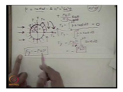
So therefore, we see that the force in the y direction, force per unit length of the cylinder in that per unit length of the cylinder the net force in the y direction is minus rho u gamma. This minus sin means the force is on the downward direction. So, the sin convention comes from from the relative direction sin of the rectilinear flow and the irrotational vortex. Here, we have considered the irrotational vortex positive in anti clockwise direction.
