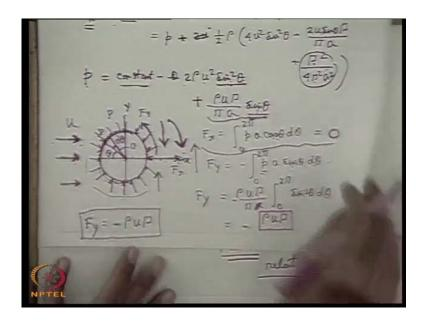
So, the net result is that if there is a circulation, how this circulation is added? Now, I tell you that this circulation is added if we have seen that if we combine rectilinear flow with the doublet we get the parallel flow past a cylinder.
