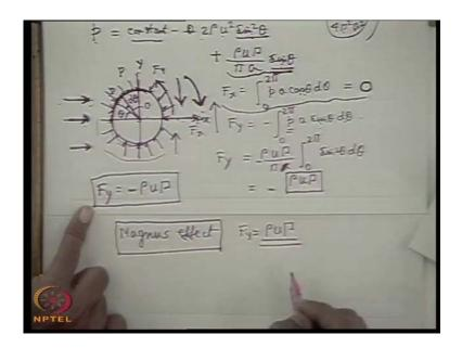
So, this phenomenon is known as Magnus effect. Magnus effect that means if we add a circulation in a cylinder flow past a cylinder, parallel flow past a cylinder then a transverse force is observed that means the cylinder is deflected transversely because of this transverse force is observed. That is the force in the perpendicular direction to the direction of flow which is known as the Magnus effect.
