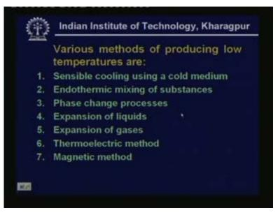
So let us look at some of the methods of achieving low temperatures the various methods of producing low temperatures are sensible cooling using a cold medium endothermic mixing of
