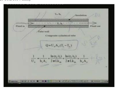
This also very commonly encountered. So here what we have is a metallic tube okay. This is the metallic tube through which a fluid is flowing okay. And this is an insulated tube so outside you
