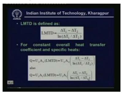
So we have LMTD introduced and it is very widely used in heat exchanger design. So this LMTD is defined as LMTD is equal to delta T one minus delta T two divided by l n delta T one by delta T two where delta T one and delta T two are the temperature differences between the hot and cold streams at the inlet and outlet respectively. So one can be inlet then two will be outlet or vice versa okay.
