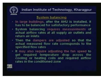
Next let us look at system balancing very briefly what do you mean by system balancing in large buildings after the air handling unit consisting of ducts coils etcetera is installed it as to be balanced for satisfactory performance. So what do you mean by balancing system balancing requires measurements of actual flow rates at all supply air outlets and return air inlet. So you have to do elaborate measurements carry out elaborate measurements of air flow rates at all air outlet and inlets.
