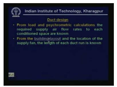
Next look at duct design normally what is the input for duct design from load and psychometric calculations the required supply air flow rates to each conditioned space are known this we have discussed earlier then from the building layout and the location of the supply fan the length of each duct run is known. For example, let me show a typical building layout.
