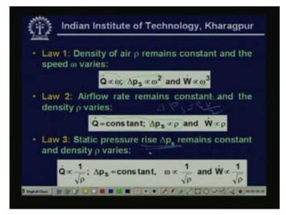
First law with law fan law one fan law one is applicable when density of air remains constant and the speed omega varies okay. So this law is valid under these conditions so when the density of air remains constant and when the speed varies from the previous relations we find that the air flow rate varies with rotative speed okay. Q dot is proportional to rotative speed that means if
