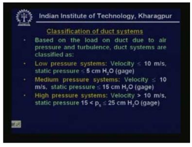
So let us first look at classification of air conditioning duct systems how they are classified based on the load on duct due to air pressure and turbulence duct systems are classified as low pressure systems.
