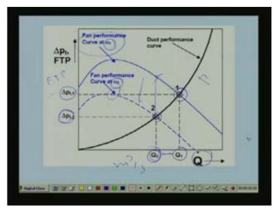
This particular curve shows the performance, fan performance curve okay. This is fan performance curve at rotative speed omega one this a fan performance curve at rotative speed omega two and this is your duct performance curve okay. Both are plotted verses air flow rate Q dot in meter cube per second right. As I said the duct performance curve is a parabolla and fan
