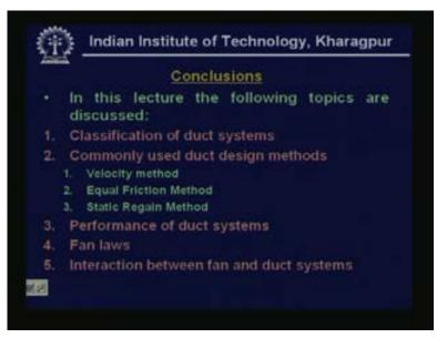
In this lecture the following points are discussed classification of duct systems commonly used duct design methods. That is velocity method equal friction method and static regain method then we have also discussed very briefly the performance of duct systems. Then we have discussed fan laws and what is the use of fan laws and finally we have discussed very briefly the interaction between fan and duct systems okay. At this point I end this lecture and I continue this in the next class.
