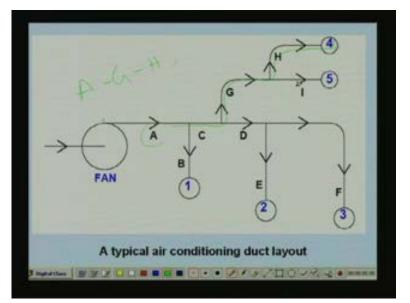
Let us say that our index run is here okay, like this let us say that means A to G to H okay, that means the pressure total pressure drop from this point to this point is the highest compared to other pressure losses okay. Pressure in the other duct runs then you call this AGH as the index run because the total pressure loss in this particular duct and is the maximum okay. So we have to select a fan which can provide this maximum pressure loss.
