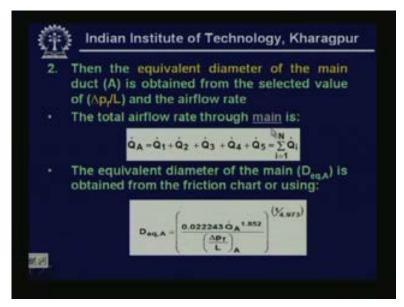
So that means delta Pf by L of duct run A is equal to delta Pf by L of duct run B that is equal to delta Pf by L of duct run C etcetera okay. Then the step wise procedure is as follows select a suitable frictional pressure drop per unit length. So that combined initial and running cost are minimized okay. So in the earlier method we have fixed the velocities where as in this method we have to select a suitable frictional pressure loss per unit length okay. That is the first step then
