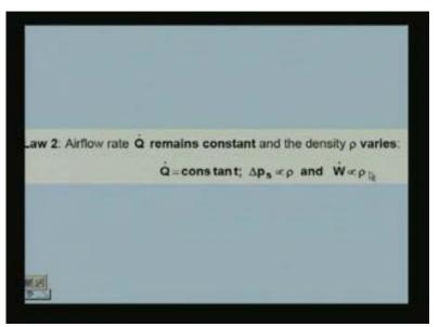
Fan law two is this air flow rate Q dot remains constant and density rho varies so and according to this law static pressure raise is directly proportional to density and power input is also directly proportional to density okay.
