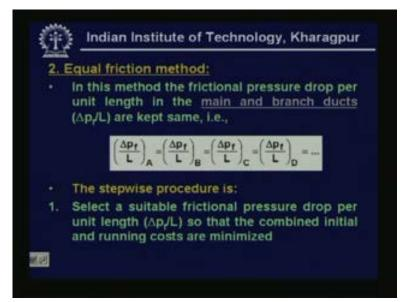
Next let us look at second method known as equal friction method in this method the frictional pressure drop per unit length in the main and branch ducts are kept same okay. That means everywhere.
