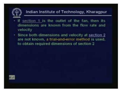
However since both dimension and velocity at section two are not known before hand we have to use a trial and error method to obtain the required dimensions of section two.
