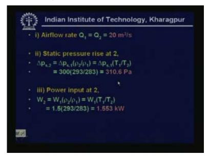
So using this you can easily find out for example air flow rate remains constant at twenty meter cube per second and static pressure raise delta Ps at condition two is directly proportional to density and density is inversely proportional to absolute temperature. So you can find out delta Ps two is equal to delta Ps one into rho two by rho one which is equal to delta Ps one into T one by T two T one T two are temperatures absolute temperatures as I said.
