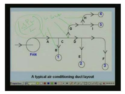
The frictional pressure drop per unit length, that means delta PF by L is constant okay, constant, for example this main for this part of the main for this branch for this branch for this branch etcetera. Every where this parameter is same this is the principle of equal friction method that is why I call it as equal friction method okay.
