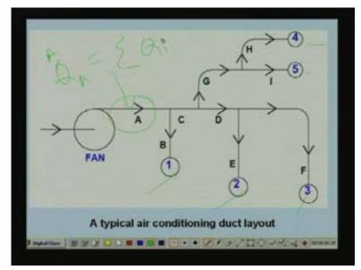
For example if you look at the figure this is the air flow rate Q dot A okay, sorry, Q dot A through this main duct run A you can see from the mass balance or volume balance that Q dot A is nothing but Q dot one plus Q dot two plus Q dot three plus Q dot four plus Q dot five okay. So this is equal to summation of different Qi's okay. So which is known to us right.
