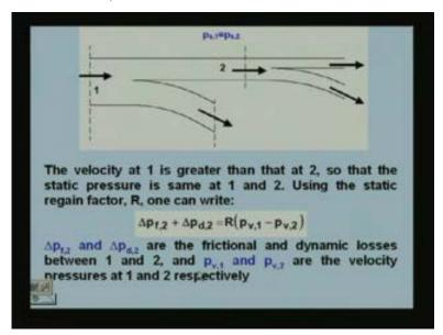
Keeping the static pressure constant before each branch or terminal okay, so this is the principle and then the total pressure drop is obtained from the pressure drop in the longest run and a fan is accordingly selected thus this step is same for all the methods okay. The fan as got to be selected finally to suit the pressure loss in the largest duct run longest duct run I am sorry, that means the duct run with the highest pressure loss okay.
