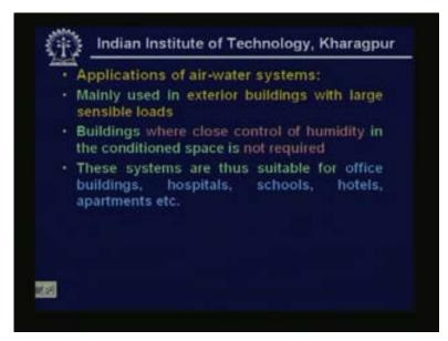
And what are the applications of air water systems they are mainly used in exterior buildings. For example for perimeter zones with large sensible loads and there also used in buildings where close control of humidity in the condition space is not required. That means if want close control of humidity you cannot use this system and these systems are thus suitable for office buildings, hospitals, schools, hotels, apartments etcetera.
