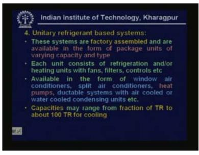
Now let us look at what is known as a unitary refrigerant based systems these systems are factory assembled and are available in the form of packaged units of varying capacity and type each unit consist of refrigeration. And are heating units with fans filters controls etcetera. And these systems are available in the form of window air conditioners split air conditioners air to air heat
