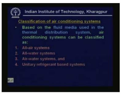
Now let us look at classification of air conditioning systems based on the fluid media used in thermal distribution system. Air conditioning systems can be classified as all air systems, all water systems, air water systems and unitary refrigerant based systems.
