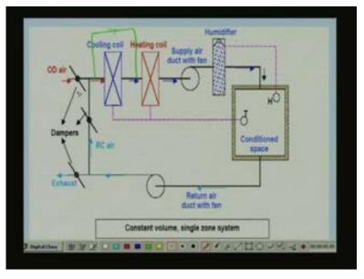
So first let us look at single duct constant volume. Single zone systems as the name implies here, we have a single duct. So through the duct either cold or hot air flows through the supply duct but both do not flow at the same time. That means you do not have simultaneous flow of cold or hot air. Either cold air flows or hot air flows at a given time and the volumetric flow rate of supply air is always maintained constant. That is why you call this as constant volume systems okay.
