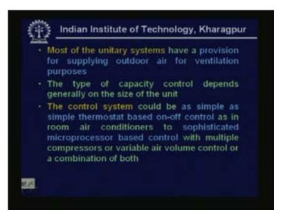
Most of the unitary systems have a provision for supplying outdoor air for ventilation purposes the type of capacity control depends generally on the size of the units and the control system could be as simple as simple thermostat based on off control as in room air conditioners to sophisticated micro processor based control with multiple compressors or variable air volume control or a combination of both okay. So the type of control system mainly depends upon the size of the system.
