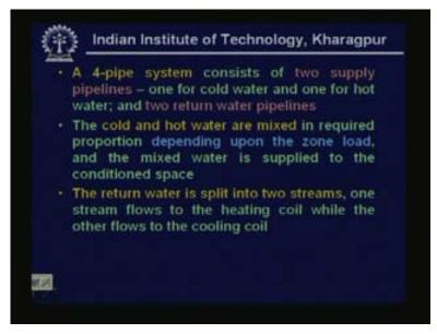
A four pipe system consists of two supply pipe lines one for cold water and one for hot water okay. In a two pipe system we just add one supply line and one return line whereas in a four pipe system you have two supply lines and two return lines okay. Two supply lines are for one for cold water and one for hot water and two return water pipe lines carry water to heating coil and cooling coil okay. That is why you call it as four pipe systems the cold and hot water are mixed
