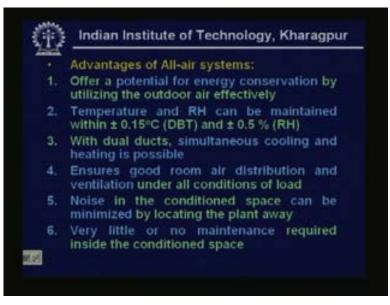
Now let us look at advantages of all air systems. All air systems offer a potential for energy conservation by utilizing the outdoor air effectively. As I have mentioned just now and temperature and relative humidity can be maintained very precisely. That means temperature can
