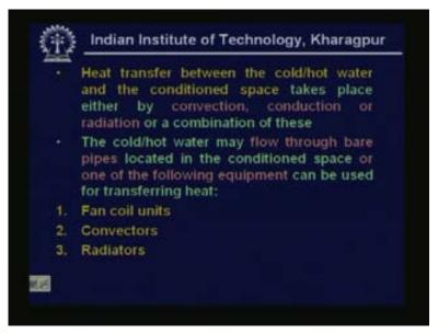
Now heat transfer between the cold and hot water and the conditioned space takes place either by convection conduction or radiation or a combination of these. The cold or hot water may flow through bare pipes located in the conditioned space or one of the following equipment can be used for transferring heat okay. That means the room units can be either a fan coil unit a convector or a radiator.
