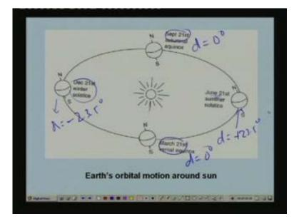
As I said, this is the orbital motion of earth around the sun and this is the summer solstice that is on June twenty-first on June twenty-first. As I said for northern hemisphere your angle of declination is plus twenty-three point five degrees and on September twenty-first and on March twenty-first. That means at the two equinoxes the declination is zero degrees okay.
