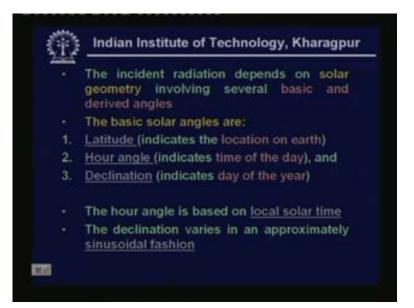
Now the incident radiation depends on solar geometry involving several basic and derived angle. So it is important to understand these angles and what are the basic solar angles the basic solar angles are the first one is what is known as latitude and the latitude indicates the location on earth. So what is this latitude?
