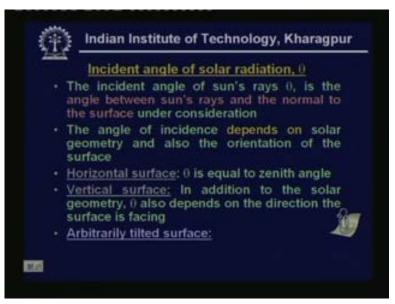
Now let us look at incident angle of solar radiation that is theta. So as I have already mentioned the angle incident angle of sun's rays theta is angle between sun's rays and normal to the surface under consideration the angle of incidence theta depends on solar geometry and also on the orientation of the surface. For example let us look at the horizontal surface theta is equal to zenith angle this can be shown very easily if you look at this figure.
