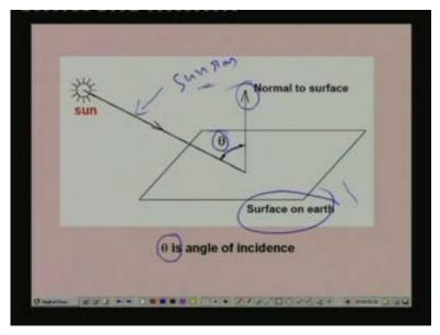
You can see that the angle of incidence is nothing but the, this is the sun's rays okay. This is your sun ray okay. And this is the surface on earth you can see here and this is a normal to the surface okay. So the incident angle is theta, theta is nothing but the angle between the sun ray and the normal to the surface okay. So this is this angle right.
