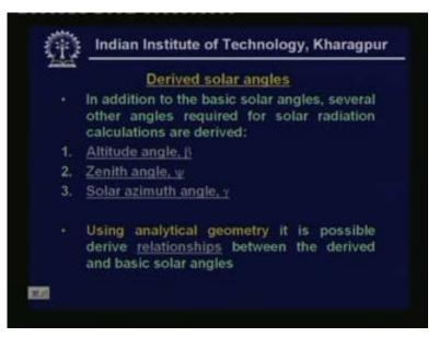
Now let us look at derived solar angles in addition to the basic solar angles several other angles required for solar radiation calculations are derived first one is what we known as altitude angle. So let us see what is this altitude angle.
