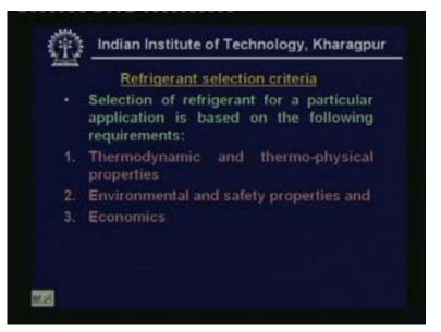
Let us look at refrigerant selection criteria selection of refrigerant for a particular application is based on the following requirements. The first requirement is thermo dynamic and thermo-physical properties. Second requirement is environmental and safety properties and finally the third requirement is economics.
