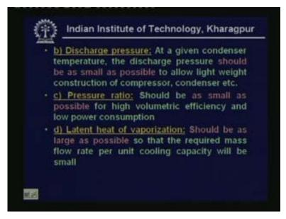
The second requirement discharge pressure at a given condenser temperature. The discharge pressure should be as small as possible to allow light weight construction of compressor condenser etcetera. So unlike suction pressure at a given condenser temperature discharge pressure should have a obviously be as low as possible okay. This
