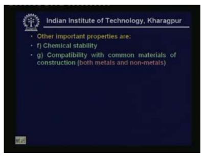
Second requirement is the compatibility with the common materials of construction. The common materials of construction are both metallic metals as well as non metals. This is a very important practical requirement the refrigerant that we use should be compatible with all materials of construction such as materials used for constructing heat exchangers various shields used in the system. Various plastics used in the system etcetera okay. It should not react with any of these materials okay.
