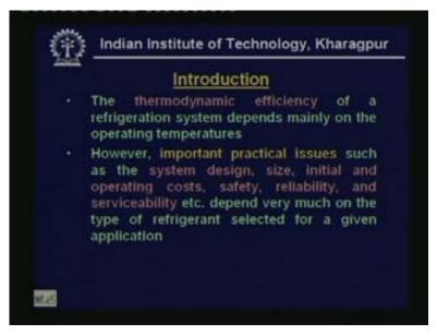
Let me give a brief introduction. You know that the thermodynamic efficiency of a refrigeration system depends mainly on the operating temperatures. That means the heat source and sink temperatures. However important practical issues such as the system
