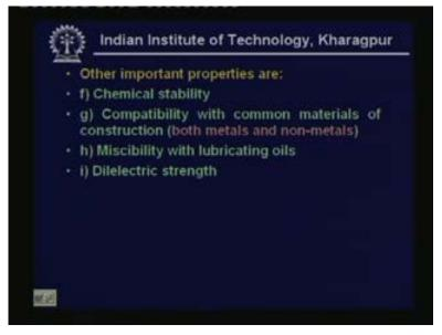
Then dielectric strength dielectric strength is very important in systems using hermetic compressors. We know that in hermetic compressors the refrigerant comes in contact with the winding electric winding of the motor okay. So the dielectric strength of the refrigerant should be high. So that it will not break down okay. This is not very important when you are talking about open type of compressors okay.
