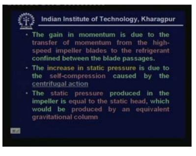
Now let me explain the physics the gain in momentum is due to the transfer of momentum from the high-speed impeller blades to the refrigerant confined between the blade passages. The increase in static pressure is due to the self-compression caused by the centrifugal action. I will explain what it is and the static pressure produced in the impeller is equal to the static head which would be produced by an equivalent gravitational column.
