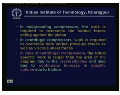
Forces acting again as the piston so why do we require work input in reciprocating compressors if you think about the working principle of a reciprocating compressor when you
