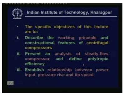
So specific objectives of this particular lecture are to describe the working principle and constructional features of centrifugal compressors, present an analysis of steady-flow compressors and define polytropic efficiency, establish relationship between power input pressure rise and tip speed.
