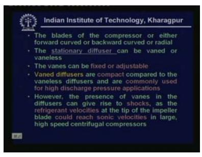
The blades of the compressor or either forward curved or backward curved or radial that mean in principle you can have either forward curved blades or radial curved blades or backward curved blades in the older machines mainly backward curved blades were used. But now-a-days the modern trend is to use radial curved blades the stationary diffuser can be vaned or vaneless I have explained that you have a component called diffuser.
