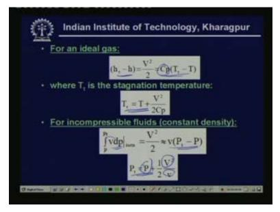
ht minus h as you know the enthalpies of an ideal gas depend only on temperatures. So ht minus h can be written as Cp into Tt minus T where Tt is the stagnation temperature and T is the static temperature here we are assuming that the Cp is constant or you are using a constant average specific heat okay. So you can write ht minus h as Cp into Tt minus T and this as you know is equal to V square by two.
