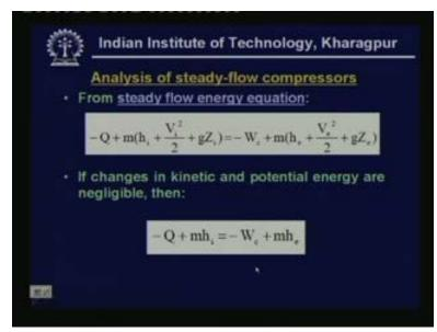
Now let us look at the analysis of steady-flow compressors this analysis is very simple analysis and it holds good for any steady-flow compressor not necessarily centrifugal compressor okay. So but we confine ourselves to centrifugal compressors in this particular lecture okay. And what we do in this analysis we simply apply the steady-flow energy equation to a steady-flow device that is nothing but the steady-flow compressor okay. So from steady-flow energy equation.
