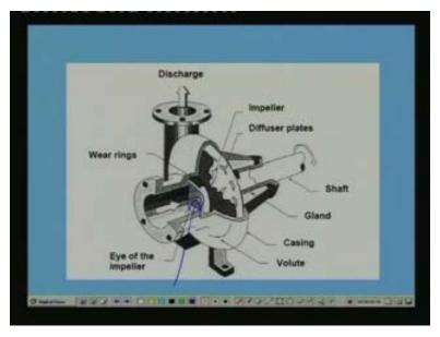
Of course you can also see the guide vanes here. So these are the guide vanes okay. So normally almost all centrifugal compressors use this guide vanes as a means of controlling the capacity okay, whereas the diffuser may or may not have vanes.
