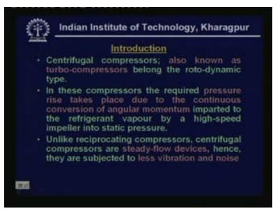
Let me give a brief introduction. As you know centrifugal compressors also known as turbocompressors belong to the roto-dynamic type. In these compressors the required pressure rise takes place due to the continuous conversion of angular momentum imparted to the refrigerant vapour by a high-speed impeller into static pressure. Unlike reciprocating compressors centrifugal compressors are steady-flow devices. Hence they are subjected to less vibration and noise.
