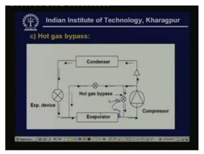
Normally this value is controlled by sensing the pressure here. That means you will be sensing the pressure at the evaporator and that is connected to this value when this pressure falls below the design pressure. That means the load is less and this value opens and once this value opens then there will be bypass and the refrigerant capacity also reduces to meet the load okay. So this is one method of hot gas bypass you can also have another hot gas bypass method where instead of sending this.
