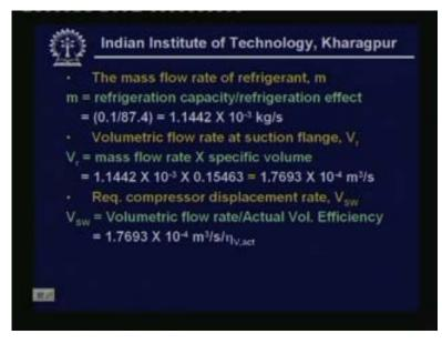
So let us solve this problem from the given input data first up all. Let us find out the mass flow rate of refrigerant as you know the mass flow rate of refrigerant is given by refrigeration capacity
