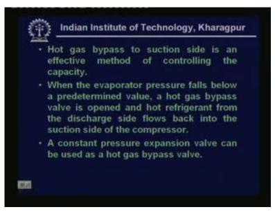
Hot gas bypass to suction side is an effective method of controlling the capacity when the evaporator pressure falls below a predetermined value a hot gas bypass valve is opened. And hot refrigerant from the discharge side flows back into the suction side of the compressor as I have already explained. And a constant pressure expansion valve can be used as a hot gas bypass valve.
