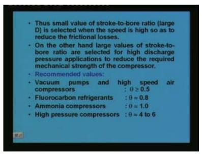
So as the result we normally find that a small value of stroke-to-bore ratio that means large D is selected when the speed is high so that we can reduce the frictional losses okay. And on the other hand when large values of stroke-to-bore ratio that means small diameter is selected one high discharge pressure applications are encountered okay. That means for high discharge pressure application you have to go for small diameter and for high speed applications you have to go for
