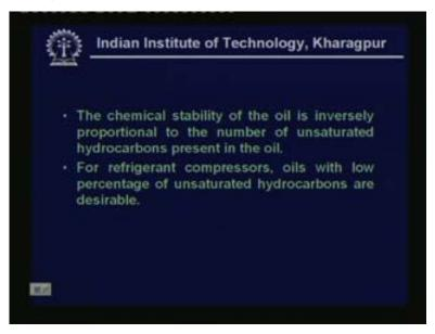
So the chemical stability of the oil is inversely proportional to the number of unsaturated hydrocarbons present in the oil. That means higher the number of unsaturated hydrocarbons smaller is the chemical stability. So for refrigerant compressors oil with low percentage of unsaturated hydrocarbons are desirable.
