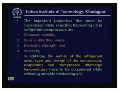
This is a very critical parameter and the important properties that must be considered while selecting lubricating oil in refrigerant compressors are chemical stability pour or floc points dielectric strength and viscosity. In addition we also have to consider the nature of the refrigerant used type and design of the compressor evaporator and compressor discharge temperatures while selecting suitable lubricating system.
