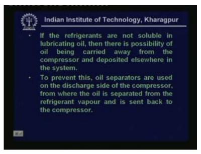
Okay, if the refrigerants are not soluble in lubricating oil then there is the possibility of oil being carried away from the compressor and deposited elsewhere in the system. This is another important problem. If the refrigerant is not soluble then oil will be carried out okay. Out of the compressor in such cases we have to use what is known as oil separators at the on the discharge side of the compressors okay. From where the oil is separated and sent back to the compressor.
