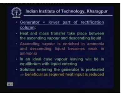
So that what I have summarised here heat and mass transfer take place between the ascending vapour and descending liquid. And ascending vapour is enriched in ammonia and descending liquid becomes weak in ammonia and in an ideal case
