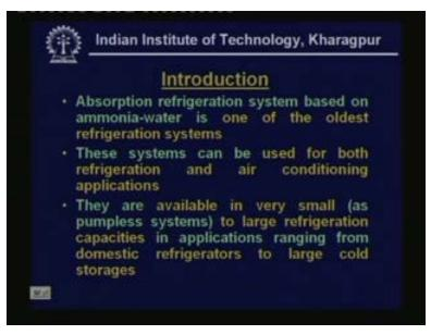
So let me give a brief introduction absorption refrigeration systems based on ammonia water where one of the oldest refrigeration systems which was developed at the end of
