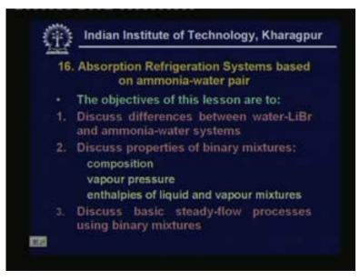
The specific objectives of this particular lesson are to discuss differences between water lithium bromide and ammonia water systems and discuss properties of binary mixtures with reference to composition vapour pressure enthalpies of liquid and vapour mixtures and finally discuss some basic steady-flow processes using binary mixtures. (Refer Slide Time: 01:26)
