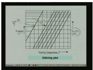
What I have shown here is known as Duhring's plot here you have solution temperature on xaxis and the saturated temperature of pure water on one y-axis and you also have on the left hand side of the y-axis the vapour pressure okay. And you can notice here that the x-axis that is the solution temperature is linear. Similarly the saturation temperature is also the scale is linear whereas the vapour pressure scale is non linear you can see that the difference is varying okay.
