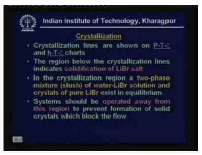
So as I mentioned the region below the crystallization lines indicates solidification of lithium bromide salt. In fact it is called as slushy region. Because in this particular region you have a two phase mixture which is a slush of water- lithium bromide solution and crystals of pure lithium bromide and they exist in equilibrium. And system should be operated away from this region to prevent formation of solid crystals which block the flow.
