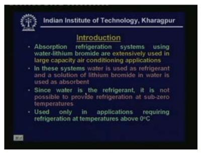
Let me give a brief introduction absorption refrigeration systems using water-lithium bromide are extensively used in large capacity air conditioning applications. In these systems water is used as refrigerant and a solution of lithium bromide in water is used as absorbent since water is the refrigerant. It is not possible to provide refrigeration at sub-zero temperatures as a result these systems are used in applications where the refrigeration temperature is above zero degree centigrade.
