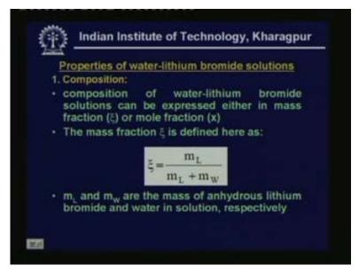
First let us look at properties of water lithium bromide solutions the first important property is composition of water- lithium bromide solutions. As I mentioned in the last class can be expressed either in mass fraction zeta or mole fraction x and the mass fraction zeta is defined here as the ratio of mass of anhydrous lithium bromide to the total mass of the solution here mL is the mass of anhydrous lithium bromide.
