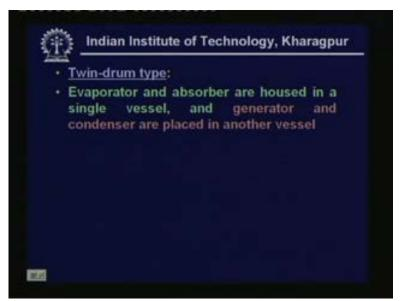
Okay, twin drum type system in this system evaporator and absorber are housed in a single vessel and generator and condenser are placed in another vessel okay. So as the name implies this system consisting consist of two drums and one drum or one vessel houses. Both the evaporator and absorber and the other drum houses. Both the generator and the condenser Okay. This is possible because evaporator and absorber operate at the same pressure almost a same pressure similarly the generator.
