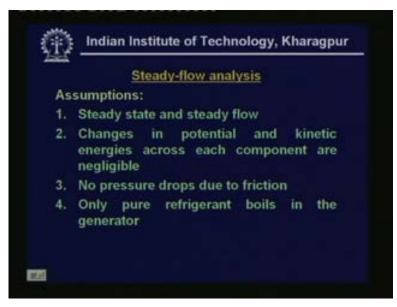
Now let us look at steady flow analysis of a simple stage vapour absorption refrigeration system based on water- lithium bromide and first. Let me list out the assumptions made the first assumption is usual assumption. It is a steady state and steady flow process then changes in potential and kinetic energies across each component are negligible. And there are no pressure drops due to friction and finally only pure refrigerant boils in the generator.
