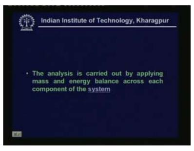
And the analysis is carried out by applying mass and energy balance across each component of the system. So let me first explain the system and let me give me give the equations.
