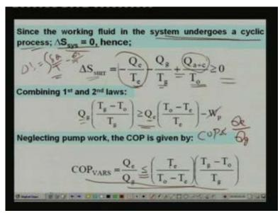
Now as I said delta S system is zero because this system undergoes a cyclic process okay. Now we write the expression for delta S surroundings means we have three temperature reservoirs one is the low temperature reservoir T e the other one is at high temperature reservoir T g and this is
