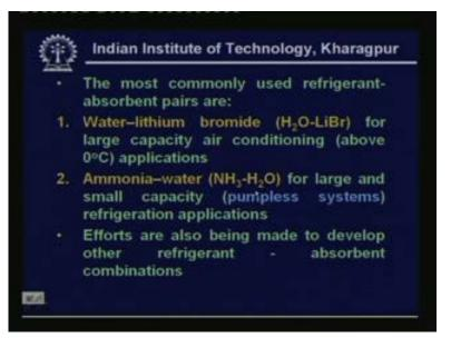
And based on these desirable properties there are two most commonly used refrigerant absorbent pairs they are water lithium bromide for large capacity air conditioning applications and ammonia water for large and small capacity refrigeration applications. So we will be discussing these systems in details in next class one or two lectures okay. And there are also other refrigerant absorbent pairs which are in at research level they are not yet commercialized okay.
