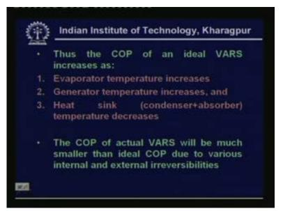
So you can see that, so from this you can easily infer that the COP of an ideal vapour absorption system increases as the evaporator temperature increases as the generator temperature increases and the heat sink temperature decreases. When generated temperature increases and heat sink temperature decreases the heat engine efficiency increases okay. And similarly when the evaporator temperature increases and the condenser temperature reduces the COP of the Carnot refrigerant cycle increases.
