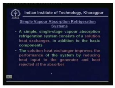
Now let us look at simple vapour absorption refrigeration systems. A simple single stage vapour absorption refrigeration system consists of a solution heat exchanger in addition to the basic components. The solution heat exchanger improves the performance of the system by reducing
