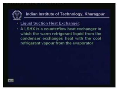
Okay liquid suction heat exchanger is basically a counter flow heat exchanger in which the warm refrigerant liquid from the condenser exchanges heat with the cool refrigerant vapour from the evaporator. So let me show this.
