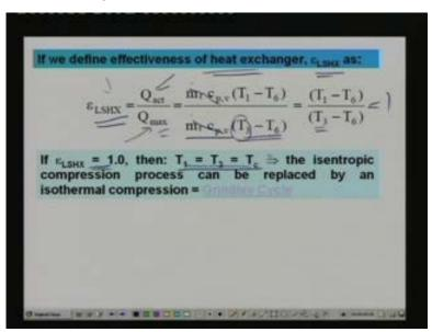
Now if you define the effectiveness of heat exchanger as the heat actual heat transfer divided by maximum possible heat transfer okay. That means I am defining an effectiveness of heat exchanger epsilon L S H X which is defined as the ratio of actual heat transfer to maximum
