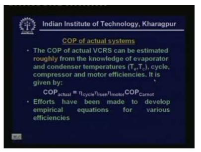
Now COP of actual systems can be given by the simple expression which is a multiplication of efficiency of the cycle efficiency of the compressor efficiency of the motor into COP of the Carnot cycle okay. This is a very rough if for a very rough estimation okay. And empirical equations have been developed to estimate the efficiency of the cycle efficiency of the motor compressor etcetera. Okay, using these equations you can get a rough idea of the actual COP compare to the Carnot COP.
