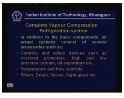
Now a complete vapour compression system in addition to the basic components consists of several other accessories will discuss this later. They are controls and safety devices such as overload protectors high and low pressure cutouts oil separators etcetera. And temperature and flow controls and filters driers valves etcetera okay. So actual system will have a lot many components over and above the basic components okay.
