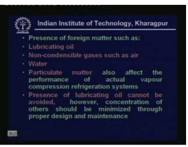
Then apart from this you can also have presence of foreign matters such as lubricating oil non condensable gases such as air and water okay. And you can also have particulate matter if you are not your system is not clean in the beginning and all these things will affect the performance of the actual systems. And the presence of lubricating oil cannot be avoided but presence of other things like air water and particulate matter has to be minimized through proper design and maintenance.
