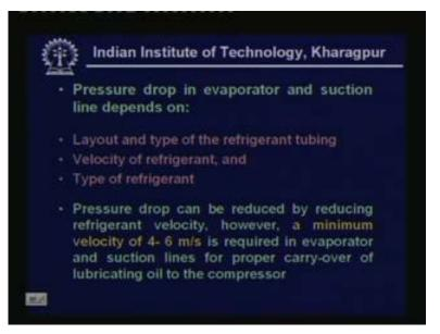
Now pressure in evaporator and suction line depends on lay out and type of the refrigerant tubing. Velocity of refrigerant and type of refrigerant and pressure drop can be reduced by reducing refrigerant velocity. However a minimum velocity of four to six meters is required in evaporator and suction lines for proper carryover of lubricating oil to the compressor. That means you have to maintain certain minimum velocity okay, even though reduction in velocity reduces the pressure drop.
