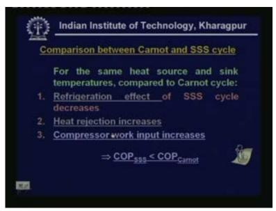
Now because of the differences in refrigeration effect and heat rejection rate we find that the compressor work input increases when you change over from Carnot cycle to standard vapour compression cycle again with the help of T s diagram, we can show this one.
