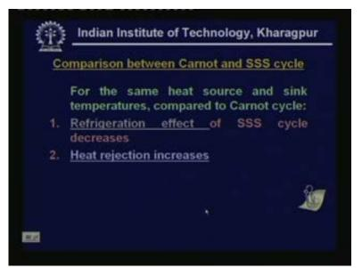
Now let us look at the heat rejection you if you find the same heat source and sink temperatures compare to Carnot cycle the heat rejection increases in a standard a vapour compression refrigeration cycle again with the help of the T s diagram. This can be shown very easily.
