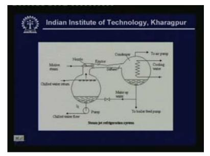
Let me explain the working principle of this. This is a typical steam jet refrigeration system. What we have here is an evaporator drum and a condenser drum. So this is the condenser drum and this is an evaporator drum. This evaporator drum consists of water. And this condenser drum also consists of water. And the motive force are the prime energy input to this system is in the form of motive steam. Motive steam means high pressure steam.
