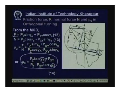
Now the friction force, this is the friction force and this is a force normal to the friction force acting at the chip tool interface. These are acting at the chip tool interface here this friction force and normal force and the ratio between these two is the apparent coefficient of friction at the chip tool interface. This is also important information to be developed for research and other purposes to study the condition etcetera.
