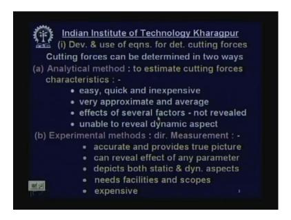
Now (i) development and use of equations for determining cutting forces being target is to determine the magnitude of the cutting force. Cutting forces can be determined in two ways;
