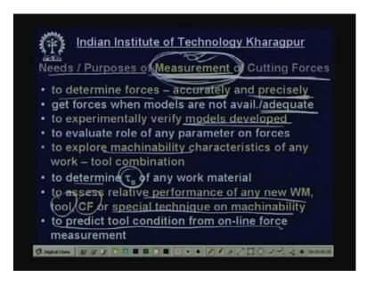
Now comes to measurement. You remember that cutting forces can be determined in two ways. Two means one is analytical method very easy, quick and inexpensive but not very accurate.
