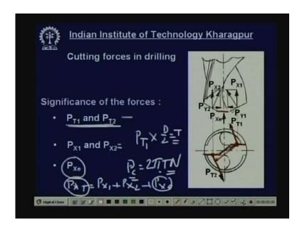
As I told you the drilling drill is a cutting tool which has got two main cutting edges. This is one main cutting edge. This is another main cutting edge connected by one small chisel edge
