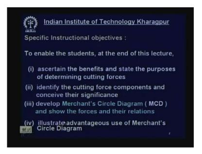
(i) ascertain the benefits and state the purposes of determining cutting forces. Why we should learn cutting force, why we should like to know the cutting forces, what is the utility? (ii) identify the cutting force components and conceive their significance in machining. (iii) develop Merchant's Circle Diagram (MCD) and show the forces content into that and (iv) illustrate advantageous use of Merchant's Circle Diagram.
