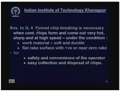
forced chip breaking is necessary when continuous chips form and come out very hot sharp and at high speed that is very dangerous under the condition work material is soft and ductile. Flat rake surface with the positive or favorable right angle for why it is given forced chip break is necessary safety and convenience of the operator, easy collection and disposal of chips.
