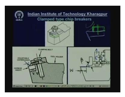
There are three types of clamped type chip breakers. As I told you that in clamped type chip breakers, this is the cutting tool flat like, and then a separate piece is fixed and clamped here. So when the chip will flow, the chip will be obstructed the flow chip will obstructed by the heel of the clamped chip. Now here you see that, this is the cutting tool. This is the cutting tool and the upper one is the chip for chip breaker.
