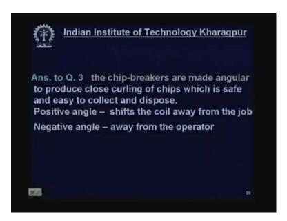
Answer to third question. The chip breakers are made angular to shift the chips either away from the operator or away from the job according to the necessity and finally the
