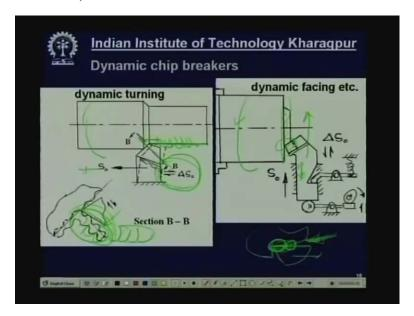
Now let us discuss something about dynamic chip breakers. What is dynamic chip breaker? It is very interesting. There is a process called dynamic turning. It is a special technique really. What is the special technique? Suppose this is the cutting tool is the tuning simple strict turning process and the chip this is the federation and this is the cutting direction. Now this is the cutting velocity and this is the feed direction.
