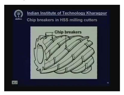
Now this is applied to milling cutter, in milling cutters, slab milling cutter and also in case of broaching cutters. Now here you see the milling cutters and this is a helical milling cutter these are the cutting edges, the fluids or the cutting edges. On the fluids the grooves are cut small grooves are cuts. Actually what happens in milling?
