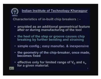
Just now you have seen in - built chip breakers. Now provided this in - built chip breakers are groove type or step or groove type provided as an additional geometrical feature like step or groove after or during manufacturing of the tool. If the cutting tools are made of high speed steel, then normally these grooves or steps are cut after manufacture of the
