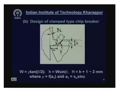
This is width W and this is the angle of the breaker and this is the radius of critical radius of curvature at which the chip is suppose to break and this angle is beta, then what we do from this geometry? From this geometry we get W. This W is equal to rho tangent of beta by two.
