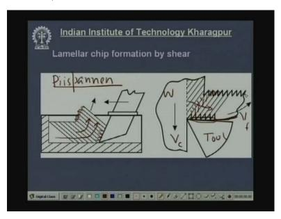
For example, suppose this is an analogy cardboard analogy. Suppose this is the stack of cardboard the post card here and now there is tool like a wooden tool. Now it has moved in this direction. It is moving in this direction, as a result these stacks will now because of this movement, these stacks will gradually this post cards will move in this direction. This will right on the rake surface of the tool and this will be like this. This will be serration.
