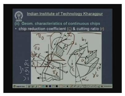
Now the geometrical characteristics of continuous chips as I told you that in machining activities most of the work material behaved ductile, engineering materials. So we concentrate on continuous chips produce by ductile materials now what are the major geometrical features of the cutting process. Chip reduction coefficient, that is chip reduction coefficient and denoted by zeta chip reduction coefficient or cutting ratio denoted by r.
