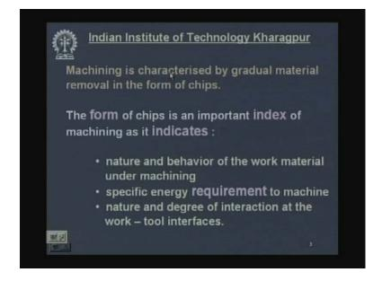
Now machining is characterized by gradual material removal in the form of chips. This has been described in detail and the purpose of machining is to provide dimensional accuracy and surface quality to the preformed blanks, to enable the object fulfill the function requirement of the object, work better, perform better and render longer service life.
