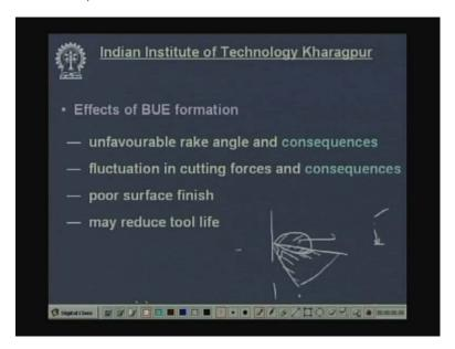
So the cutting tool will quickly lose material by damage and its life will decrease.
