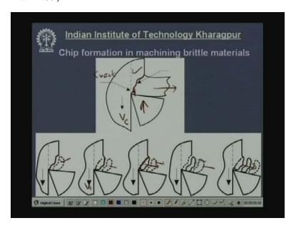
Now come to chip formation in machining brittle materials it is a different process now chip formation is a permanent deformation process whether is ductile or brittle because it is the failure permanent deformation of the work material in form of chips. Ductile material are formed by what is called yielding or shear, but brittle materials are formed by brittle fracture.
