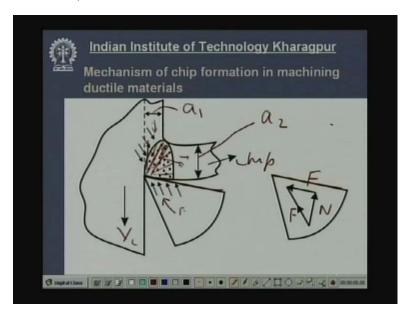
Now here let us see the mechanism of chip formation in machining ductile materials because of mechanism of machining ductile and brittle materials are entirely different widely different, but most of the materials engineering materials that a machine are ductile even if ductile they are semi brittle or semi ductile under the cutting condition they behave ductile. So most stress will be given on the mechanism of chip formation in machining ductile materials.
