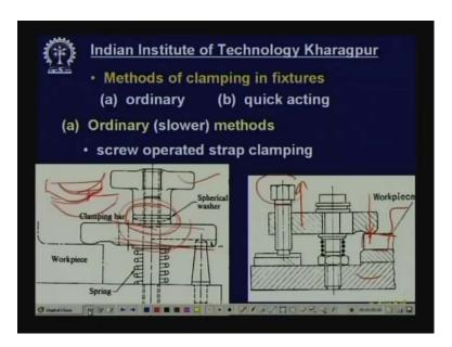
The spherical washer is like this. Spherical washer which works in another washer, which is also got one cavity like this. So this can tilt with this. So this will be taken care of. Now this is the other side, other part. So this is the screw clamping screw. If you rotate it clockwise, this strap will be raised and this will move down and apply the clamping force on this work piece, the part of the work piece on the base plate. Now clamping from side or through machining:
