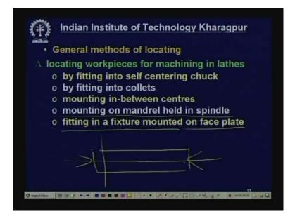
Locating work pieces for machining in lathes which are very common work by fitting in to self centering chart, by fitting in to collets, mounting in between say centre. Here is a job, you have put one centre here headstock centre tailstock centre. It will be automatically aligned. Of course, it has to be held in a position by a dog or catcher driving plate. Mounting on mandrel held on spindle. This will be shown later on and fitting in a fixture mounted on a face plate. (Refer Slide Time: 29:50)
