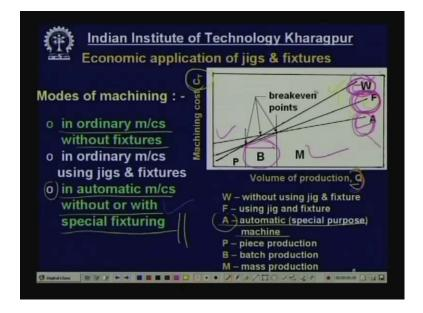
Now you can see for this batch production region, for the batch production region the bottom most line is belonging to 'F' that is jig fixture, so we can machine. Therefore it is clear that mode one is suitable economically viable for piece production or job order production, then automatic system is suitable for mass production because it is expensive and for batch production use of jig fixture is most appropriate. Now, the design of jigs and fixtures:
