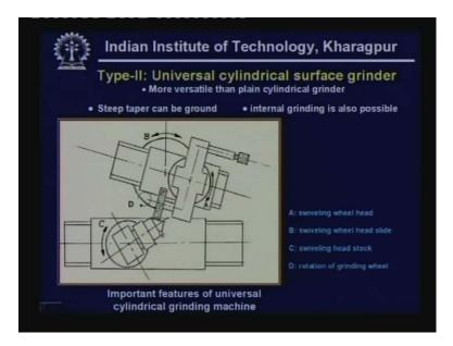
This is universal cylindrical surface grinder. Now what we have seen? In the plain surface grinder apart from straight cylindrical grinding, a small taper can also be ground just by
