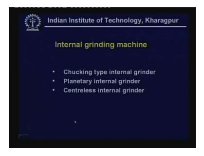
These internal grinding machines are working in the same way as machining a bore in a particular lathe. Now this internal grinding machine can be just chucking type internal grinder, we can have planetary type internal grinder or also we can have center lathes internal grinder.
