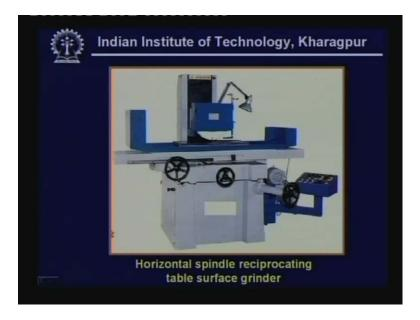
This is the actual photograph of a typical surface grinder. This is the wheel head, the column, the base, this is the work table. We can see three hand wheels one two three. This one is used for manual movement of the work table in the longitudinal direction. It can be of course automatically fit, this one this will be used for transverse moment of the work table and the third one that is to provide the down feed for the wheel this grinding wheel.
