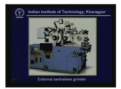
So this is the actual the picture of a center lathes grinder there we have the grinding wheel and this does not have any center support so long rods are used for grinding in this machining.
