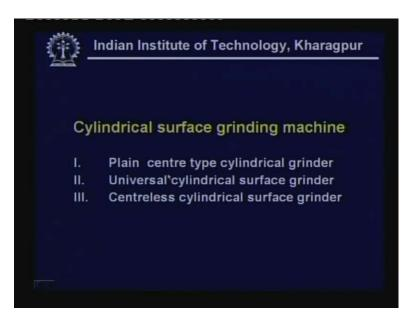
Now we go to cylindrical surface grinding machine. In cylindrical surface grinding machine, we see that at least there are three types of grinding machine. One is plain center type cylindrical grinder. Number two is universal cylindrical surface grinder and then the third one is centre less surface grinder. Now the plain center type surface grinder as we see here, this is very similar to operation just like turning in a center lathe.
