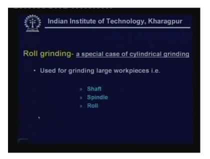
Now as an extension of this cylindrical grinding, we have also roll grinding machines. These roll grinding machines are quite large in size. These are used mainly to handle large work pieces like shaft, spindle and rolls which are used in rolling mills after machining in roll turning lathe, it needs further processing that is to achieve improved accuracy and finish and that can be easily, effectively accomplished in this roll grinding machine.
