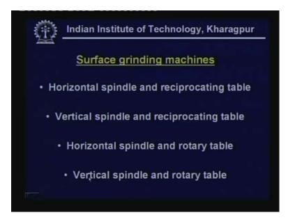
Surface grinding machines: In this particular category, at least we can see there are four machines. One is horizontal spindle and reciprocating table, the second one is vertical spindle and reciprocating table the third one horizontal spindle and rotary table and the last one vertical spindle and rotary table.
