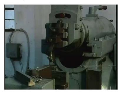
backward and the forward motion is the cutting motion that removes the chip then it comes back. After removing one strip of material, this work piece will come this side or that side and that is called feed motion. So combination of this cutting motion of the tool and feed motion of the job produce the flat surface. Now this flat surface is produced by removing the excess material from the top, that is the top layer strip by strip with help of the cutting tool in the form of chip.
