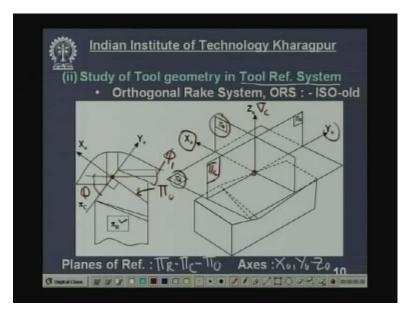
Study of Tool geometry in Tool reference system. Here, the configuration of the cutting tool is taken as a reference not the machine tool, again the tool reference system is classified into two type, orthogonal rake system symbolized ORS orthogonal rake
