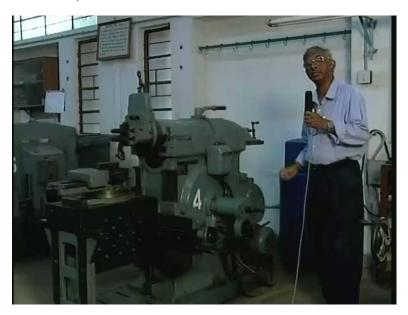
suppose this top layer has to be smoothened and flattened by removing this layer gradually. Now here the metal will be removed in the form of chips strip by strip with the help of the cutting tool. This cutting tool is mounted on the tool holder which is fixed in to the rim which is main part of the shaping machine which reciprocates forward and
