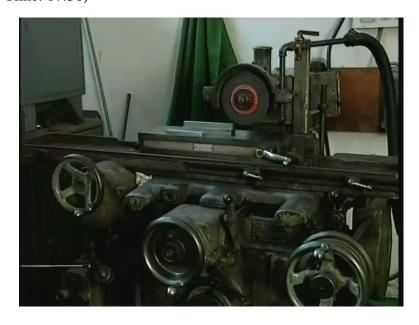
and smooth machining like shaping, milling, turning in lathe cannot produce very high accuracy and surface finish. For that, such kind of grinding operation is necessary. Grinding machines can produce flat surface, cylindrical surface and contour surface. This particular machine is called surface grinder which finishes only flat surfaces as shown over here.
