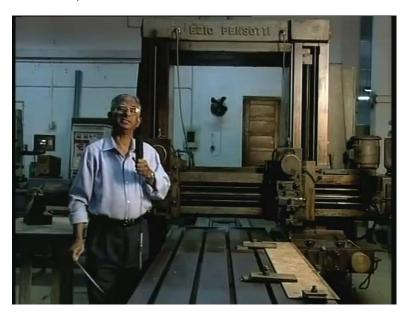
The main constructional features are - it has got a long bed, you see on which a table that will reciprocate and on the table the job will be mounted and this is the cutting tool which is mounted on the tool holder and this cutting tool moves in two directions, in horizontal direction and as well as in vertical direction. This is called the rail and this is called the frame and the operational characteristics are this produces generally flat surfaces.
