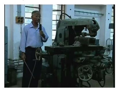
There are different types of milling machines. This is conventional milling machine and here you see, this is the cutter which is mounted on a rod like called arbor
