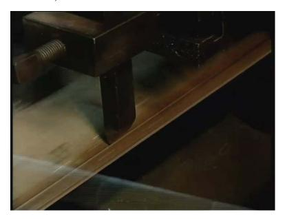
continue until the work is complete. Combination of this cutting motion and the feed motion produces what is called a flat surface. Now here in front of us, we see one machine tool called the lathe and this is the most primitive widely used common
