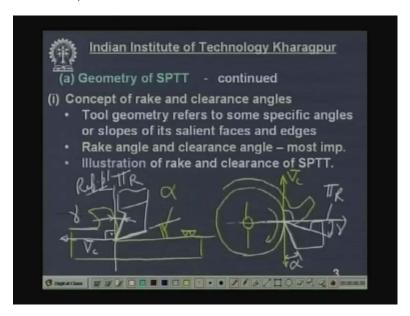
It refers to some specific angles or slopes of the cutting tools, salient faces and edges or like cutting edges rake angle and clearance angle are the most important features of the cutting tool. Now, illustration of rake and clearance of single point turning tool.
