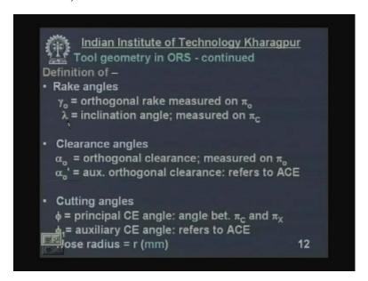
What is rake angle orthogonal rake? Orthogonal rake is measured on orthogonal plane but as such orthogonal rake means angular inclination of the rake surface from reference plane and measured on orthogonal plane then lambda inclination angle of the main cutting edge is also a rake angle, inclination angle is measured on cutting plane. Now the clearance angles. This is called orthogonal clearance of the main cutting edge.
