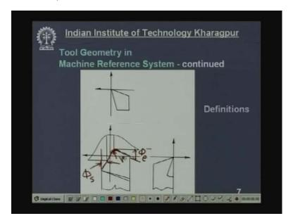
What is this angle? This is called cutting angle, this is the cutting edge main cutting edge this is the cutting angle and this is denoted by phi S. This is called approach angle angle of inclination of the main cutting edge from machine transverse plane. So this is pi Y machine transverse plane phi S and this angle is called end cutting edge angle phi e so what is the definition of approach angle this cutting angle.
