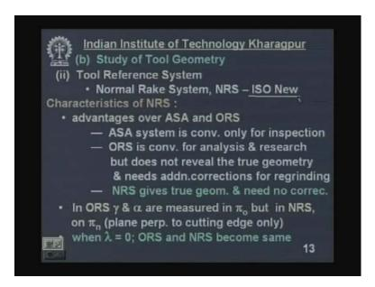
Tool Reference System are two category. One is orthogonal rake system and other one is normal rake system. This is normal rake system denoted by NRS and this is a new concept. It came recently compared to orthogonal rake system this is also called ISO New. New means may be thirty years or twenty five years. Now what are the characteristics of normal rake system over ASA system and orthogonal rake system? Let us have a look. ASA system is convenient only for inspection.
