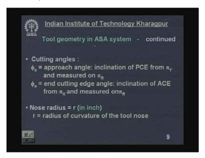
transverse plane and measured on reference plane. Both the cutting angles are measured on reference plane end cutting edge angle already defined. Now nose radius I already mentioned the purpose of radiusing the tool tip mechanically strengthen and better finish. This is expressed in inch in ASA system or machine reference system this has to be noted. Now R is the radius of curvature of the tool nose. Now come to tool reference systems.
