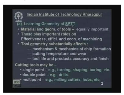
Start with learning tool geometry of SPTT that is, single point turning tool. It is simply told SPTT. Now we should remember before going to the tool geometry why it is so important. Material and geometry of cutting tools are very very important and both are equally important so far as machining, machinability, machine economy are concerned. This tool geometry and tool material plays important roles on effectiveness, efficiency and economy of machining.
