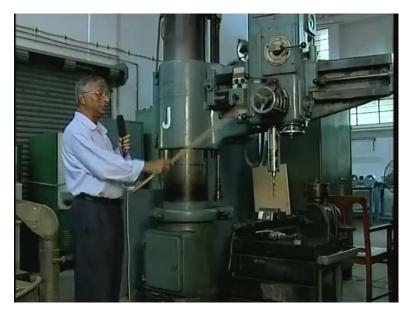
In drilling machine the main function is to make circular hole or cylindrical hole
