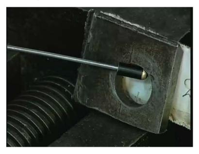
in solid body like this, which requires a cutter like this called drill or drill bit. The drilling cutter which makes the hole and this is the drill point which the main cutting
