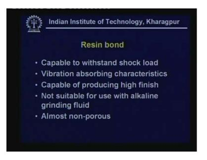
Now we have resin bond which is capable to withstand shock load vibration capacities and it is also used where we have some kind of vibration in the machine and this is also good for high grinding finish, but it is not suitable for alkaline grinding fluid.
