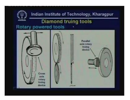
Now so for we have used a translatory tool, but here we have a rotary turning truing tool and this rotary truing tool can have cross axis or parallel axis instead it is just like a rotary tool which is doing the necessary truing action.
