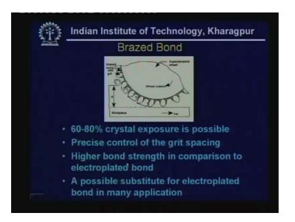
Now this is braze bond. This is an innovative approach made where we can still increase the crystal exposure and with this crystal exposure, the high material removal rate can be possible and this is going to be a substitute for electroplated bond. Now we go to the wheel conditioning section.
