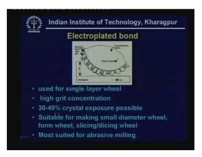
This is an electroplated bond which is used for high crystal exposure. It gives high concentration. Here single layer that is bonded suitably in a galvanic metal layer and this is used for high material removal rate for abrasive milling and so.
