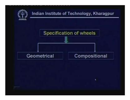
Now there are at least two types of specification. One is the geometrical specification which shows the diameter, the width and the bore of the wheel. The second one is more important that is the compositional specification which takes care of the material of the abrasive, material of the bond, its hardness, grit, spacing velocity and so on. We find here the various shape of the conventional wheel.
