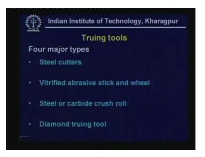
So here we have four types of truing tools, steel cutter, and vitreous abrasive stick steel crushing roll or diamond truing tool which happens to be the most efficient.
