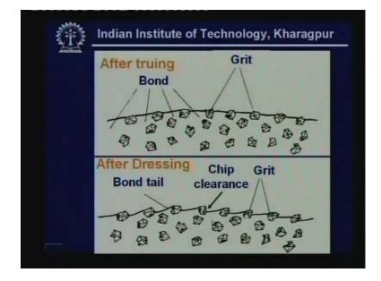
Here we can see a truing after truing operation, what we can see the bond material and the grit material that they are leveled. So this grit cannot have any cutting capacity. Now in the dressing, we have to scoop out this material to clear the space for chip clearance. Now with this chip clearance, we have enough space for grinding action. So this is actually dressing.
