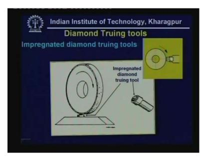
This is an impregnated wheel impregnated tool which is used for this truing action which is illustrated here.
