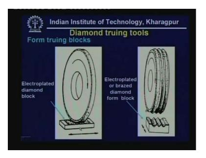
These are the two electroplated diamond blocks. This can be also used as a truing wheel and in this case these blocks can be reciprocated to have necessary truing, it is a flat truing or a form truing instead of using either a rotary tool or a single point diamond nib. So this can be done either by electroplating or by brazing.
