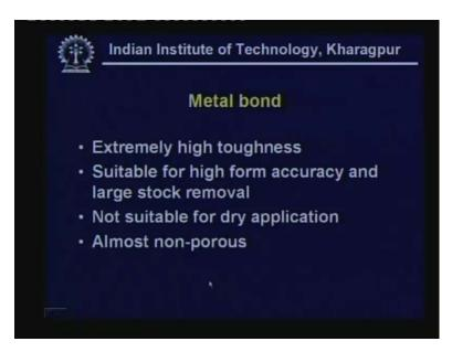
This is actually a metal bond which is extremely tough suitable for high form accuracy and large stock removal. It is almost nonporous.
