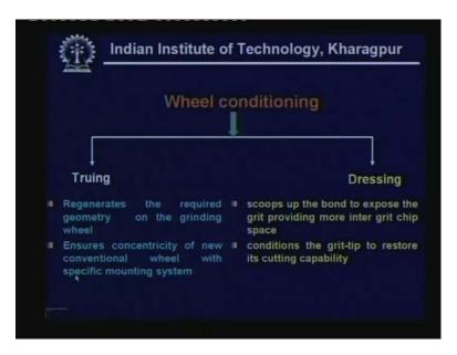
Here we have either truing or dressing. Truing means getting the macro form on the wheel and in those cases where making the spinning axis properly aligned with the geometrical axis of the grinding wheel that also comes under the purview of truing and what is dressing? Dressing means opening of the wheel, that means making the space for
