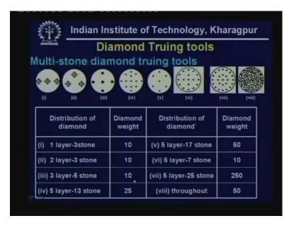
We have different types of truing tool either with a multi point this diamond or we have an impregnated diamond which is illustrated in this figure.
