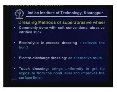
So this dressing method of superabrasive wheel which goes along with either use of a vitrified stick or we can have just electrochemical dressing where by the bond material can be electrochemically etched to have release of the protrusion of the grit material and
