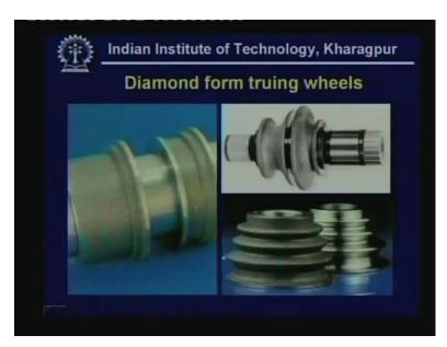
These are the actual truing wheel which can be used in practice to do necessary truing on the abrasive actual grinding wheel.
