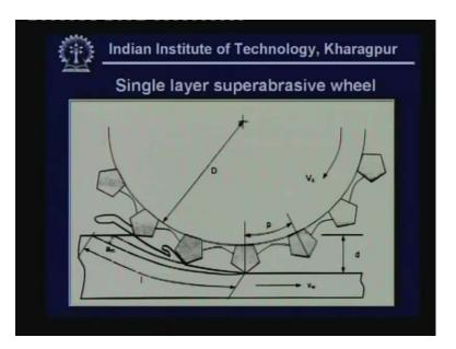
So this shows us actually the type of wheel which is a single layer type of wheel. This is a special type of bond which is illustrated in the following slide.
