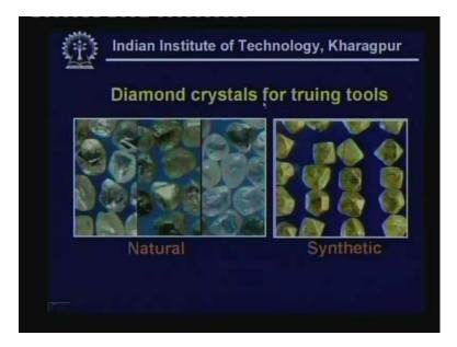
These are the different types of diamond crystals which are used for this truing tool. This is natural crystals and we have also synthetic crystals, which goes straight in the preparation of the truing wheel.
