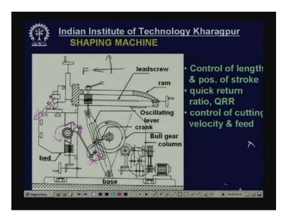
Now the amount of so this amount of movement or the rate of feed depend upon that how much angle this ratchet rotate that will depend upon the amount of oscillation. This will depend upon this radial distance which can be time to time changed this extrinsity. This is how we get automatic feed. Now by changing the pawl by 180 degree we can change the direction of rotation by changing the direction of rotation the table can be moved in this way or in this way so this is feed.
