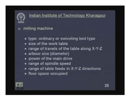
Now milling machine, type - ordinary type or swiveling bed type. The bed can be rotated slightly in addition to xyz moment size of the work piece work table range of travels of the table along x direction, y direction, z directions. Arbour size, the diameter the board diameter of the cutter will be decided by the arbuor size. Power of the main drive say kilowatt range of spindle speeds or the arbuor speeds range of table feeds in the xyz directions and floor space occupied.
