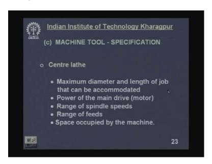
Now come to machine tools specification. How to specify machine tools? When you go to market for purchasing a lathe, you have to tell what kind of lathe you want, what amount of power, what kind of lathe, then what should be the size of the lathe, and what can and all these things you should be very clear you should very clearly mention. Otherwise you cannot purchase it procure it.
