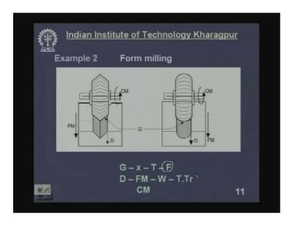
Now here you see Form milling. In this case of Form milling what we are actually producing this is the milling cutter. This shows the milling cutter and this is the work piece a chemical block in which a slot has to be cut. A group a V group has to be cut. Now we take the cutter with the V group V shape so getting this particular shape of the group metal removal. So this portion is the generatrix and now these generatrix when it travels along this path the directrix we get this slot.
