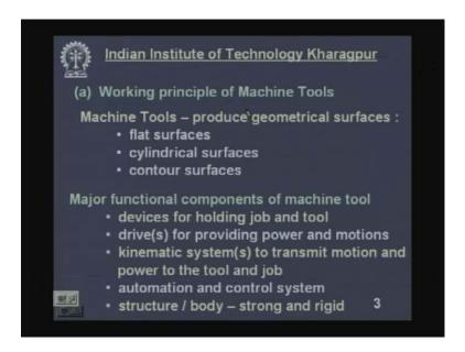
Now see the working principle of Machine Tools. I remind you the machine tools - they produce geometrical surfaces. This was mentioned in the previous class also. Now when you say geometrical surfaces we mean flat surfaces, cylindrical surfaces and contour surfaces which can be mathematically expressed and redrawn according to program. Only those will be called geometrical surfaces.
