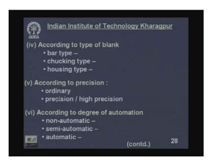
Then according to type of blank, blank may be bar type, chucking type and housing type. Housing type are generally big machine tools according to precision ordinary or precision even high precision. This way machine tools can be classified. According to the degree automation so machine tools need automation it can non automatic like centre lathes. Semiautomatic like capstan lathe, turret lathe, automatic like single spindle automatic lathe.
