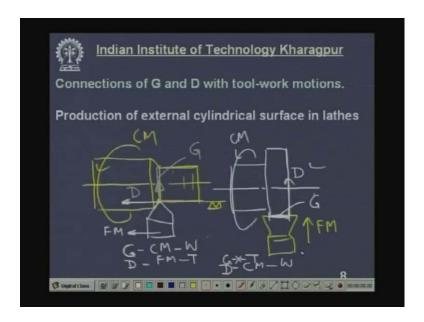
Now connections of generatrix and directrix with tool work motions production of external cylindrical surface in lathe. Now you see where the cutting motion and feed motion will be connected with the generatrix and directrix and this produces cylindrical surface. Now say there is a blank, a rod undergoing turning operation. Now what are the motions? This is feed motion. Cutting motion rotation of the job and this is cutting motion.
