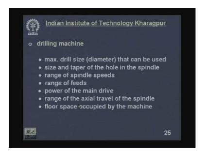
Coming to drilling machine, maximum drill size maximum is the diameter of the drill which will decide the maximum diameter of the hole that can be produced, size and taper of the hole in the
