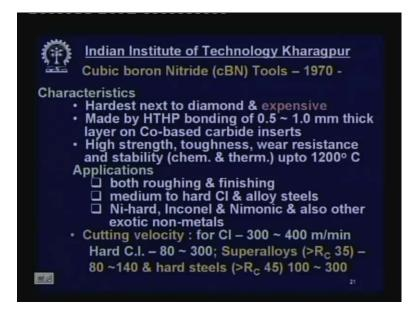
Now there are two more super materials. One is Cubic boron nitride and other one is diamond. What is Cubic boron nitride? These tool were introduced in 1970, Cubic boron
