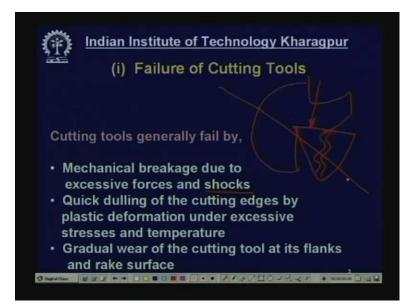
You know for smooth efficient and economic machining process to be continued the cutting tool should not be allow to fail abruptly or frequently. First of all, the abrupt or catastrophic failure of the cutting tools have to be prevented totally and the normal failure
