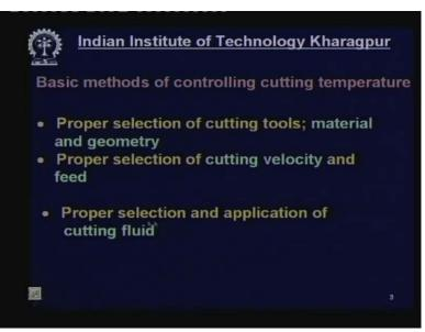
Now what are the basic methods of controlling cutting temperature? There are three basic methods .One is a proper selection of the cutting tools; the material and geometry both of
