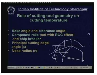
What is principle cutting edge? This is the principle cutting edge you remember that this is the cutting turning process and this angle is principle cutting edge angle. Now this principle cutting edge angle if it is less say like this, this much then temperature will be less and if it is large then the temperature will be large for example it is like this if you
