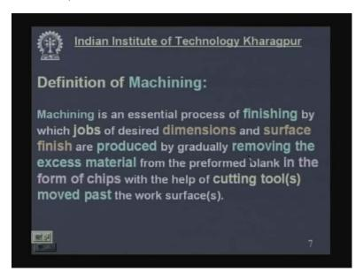
Machining is an essential process of finishing by which jobs of desired dimensions and surface finish are produced by gradually removing the excess material from the preformed blank in the form of chips, with the help of cutting tools moved past the work surface. So is essential feature of this process is the dimensions good dimensions and surface finish by removing the excess material in the form of chips with the help of cutting tool.
