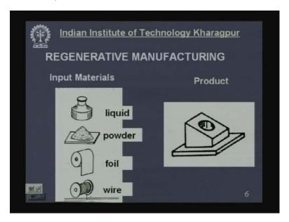
Suppose this is the product, a complicated product. This can be done by taking raw material in the form of liquid. If you take it take in the form of liquid, this is called stereo lithographic method. You can start from powder or the selective sintering process. You can start from the foil as a lobe layered manufacturing by metal and wire you can use the wire as the source of material and using the FDM process, you can gradually produce it. Now next is machining. Now let us come to machining.
