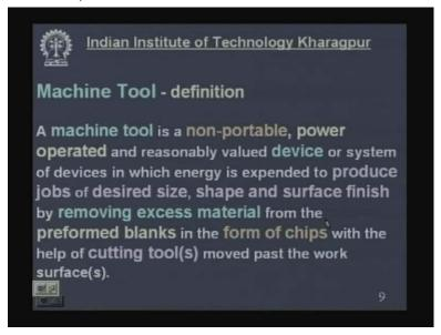
Now what is machine tool? This work has to be done in machine tool. The machine tool is a device in which the job and tool have to be formed, where it the motion and power have to be transmitted from the source of power to the tool and job. Then control of the
