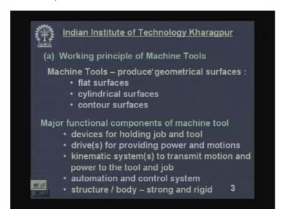
I remind you Machine Tools - they produce geometrical surfaces. This was mentioned in the previous class also. Now when you say geometrical surfaces we mean flat surfaces, cylindrical surfaces and contour surfaces which can be mathematically expressed and redrawn according to program. Only those will be called geometrical surfaces.
