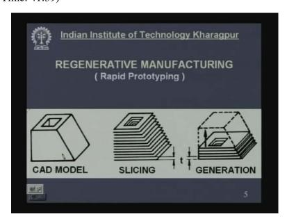
So simple example here you see that, suppose this is the product which has to be made or manufactured. A solid body of metal say brass and then first of all, this job has to be drawn properly not physically but this has to be drawn to the computer by CAD, AutoCAD or some other CAD model. So you draw this thing in a computer or you can get a solid job and then by when a proving or measuring the dimensions you can put the
