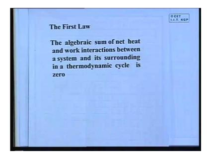
The first law is the algebraic sum of work and heat interactions, net work and heat interactions in a cyclic process by a system with its surroundings in a cyclic process is zero. Today it appears to be a common sense, because in a cyclic process when a system come backs to its initial state all the energy interactions have to be zero, it gains something, it loose something and ultimately it is net zero.
