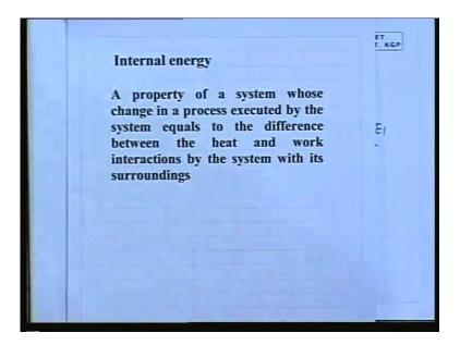
A property of a system whose change in a process executed by the system equals to the difference between the heat and work interactions by the system with its surrounding, this is
