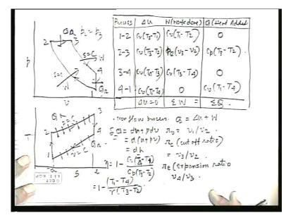
Let us draw this cycle quickly; 1, 2, 3, 4. This is the pv diagram and is important. The suction and exhaust, we are not drawing. This is Qa process, which means the heat added and heat rejected. These are the two isentropic processes. No question of heat addition and rejection. If we draw the TS diagram, it will look the same. But, to show that one is having a concept, one should do like this. This is a constant pressure process; 1-2, 2-3 then 3–4, this is a constant volume process.
