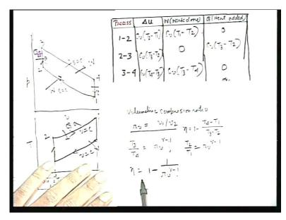
Volumetric compression ratio is denoted as  $r_v$ , which is equal to the ratio of the two volumes; that is the maximum volume to the minimum volume  $v_1$  by  $v_2$ . This is the volumetric compression ratio. We have the expression for eta is equal to 1 minus  $T_4$  minus  $T_1$  divided by  $T_3$  minus  $T_2$ .
