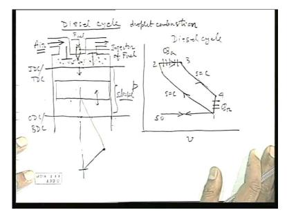
In the similar way as we started Otto cycle, Diesel cycle is again a standard cycle but this is followed in an IC engine where diesel is used and the particular engine cycle follows a compression ignition engine. That means the combustion and the admission of fuel vapor and air or fuel and air is made in a different way as done in spark ignition engine.
