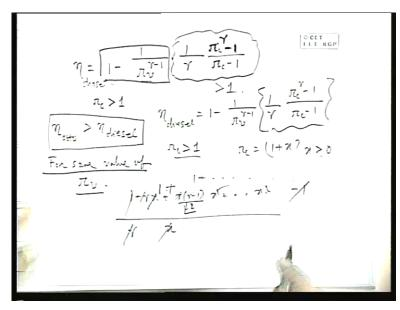
So, this part is multiplied by 1 by gamma  $r_c$  to the power gamma minus 1 divided by  $r_c$  minus 1, where  $r_c$  is the cut off ratio. Cut off ratio is this one  $r_c$  is  $v_3$  by  $v_2$ . Therefore, one can write  $r_c$  greater than 1.
