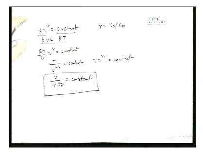
We know for an isentropic process pv to the power gamma is constant. Gamma is  $C_p$  by  $C_v$ . The equation of states pv is equal to RT, r is the characteristic gas constant, v is the specific volume.
