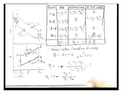
We also express the efficiency eta in terms of heat quantities. In this cycle, one very important parameter is there, which is defined as volumetric compression ratio.
