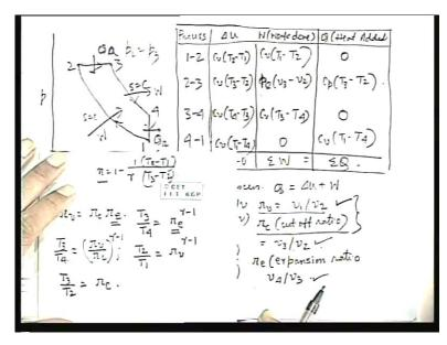
Expression for efficiency eta is 1 minus 1 by gamma. You can see that,  $T_4 - T_1$  divided by  $T_3 - T_2$ . You can write with the definition of  $r_v$ . With this definitions of  $r_v$ ,  $r_c$  and  $r_e$ , we can write  $r_v = r_c r_e$  because  $v_2$  by  $v_4$ ;  $v_1$  by  $v_2$   $v_1 = v_4$ . So, we can write,  $r_v$  is equal to  $r_c$  cut off ratio into expansion ratio.
