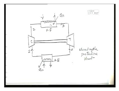
It is like this. There is a compressor and air is coming here, there is no fuel injection, that means the air is being heated from an external source that means external hot fluid comes and goes and it heats the air. This is 2, from 2 to 3 that means here the heat added is  $Q_a$ . The next part is the same that means this is the turbine part. From 3 to 4 is the turbine air, then the same air is cooled while going from 4 to 1 by a coolant.
