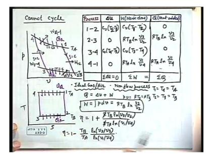
We have studied Carnot cycle in few last occasions, so we know what is a Carnot cycle. If you plot the PV diagram for Carnot cycles we will see the Carnot cycle consists of two isotherms and two isentropic so these are the two isentropic line air s is constant s is constant and this is e is T constant so this line is constant temperature line so these two lines is T is constant, T is constant so it consist of two isothermal and two isentropic.
