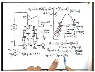
Let us consider this boiler here, and the steam enters at some pressure and temperature. The boiler pressure and temperature at this point 1 and this steam expands up to the condenser pressure 2. Let us consider point 2, which means steam after expanding to a
