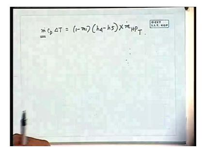
hp turbine hp m dot hp turbine. Since I will have to find out the mass flow rate of the cooling water, if you suppress it, the result is the mass flow rate of the cooling water per unit steam flowing through the hp turbine. Next part, if the velocity of steam flowing from the LP turbine to the condenser and is limited to a maximum of 130 meter per second. Find the diameter of the connecting pipe.
