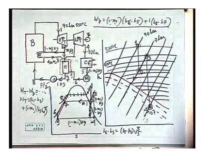
This is the boiler, this is the turbine. Now, boiler 1, which is 90 bar and 550 degree Celsius. After expansion, this is HP turbine, rather turbine T, this is LP turbine.
