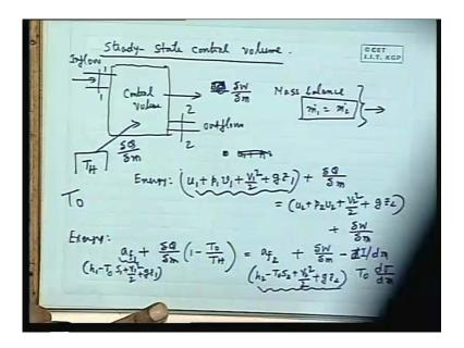
Let us consider a steady state control volume. Let me draw the diagram. So, this is inflow section one and this is outflow steady state. This is control volume which gives shaft work. When it is a steady state, I write in terms of per unit mass del W divided by del m as it is coming and let heat is added from a reservoir  $T_{\rm H}$ .
