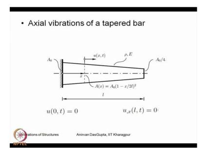
Now let us, look at this example of the tapered bar. So, as you can see, it is fixed at x is equal to zero and it is free at x is equal to l. So, the geometric or essential boundary condition is on the left boundary, where the bar is fixed. So, we must choose functions, Admissible functions, which satisfy the boundary condition at the left.
