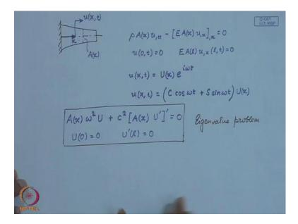
So, let us start by re-visiting the modal analysis problem. So, in our last lecture, we had discussed the problem of a bar with varying cross section. The equation of motion of the system was given by this and the relevant boundary conditions for this problem were given by U at zero is equal to zero for all time and on the right boundary we have natural boundary condition and in the order to do the modal analysis we were searching for solutions of the special form or structure.
